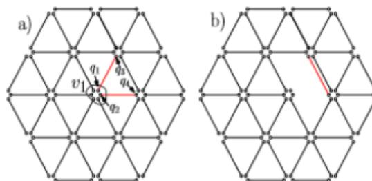
Figure 13: (Color online) a) Mapping a quantum network to a percolation problem. Qubits are represented by small circles. Each vertex (node) contains six qubits. b) using entanglement swapping to transform the lattice structure. The two red (grey) bonds in a) are replaced by the red bond in b). This process can be continued to produce a double-bond hexagonal lattice.
