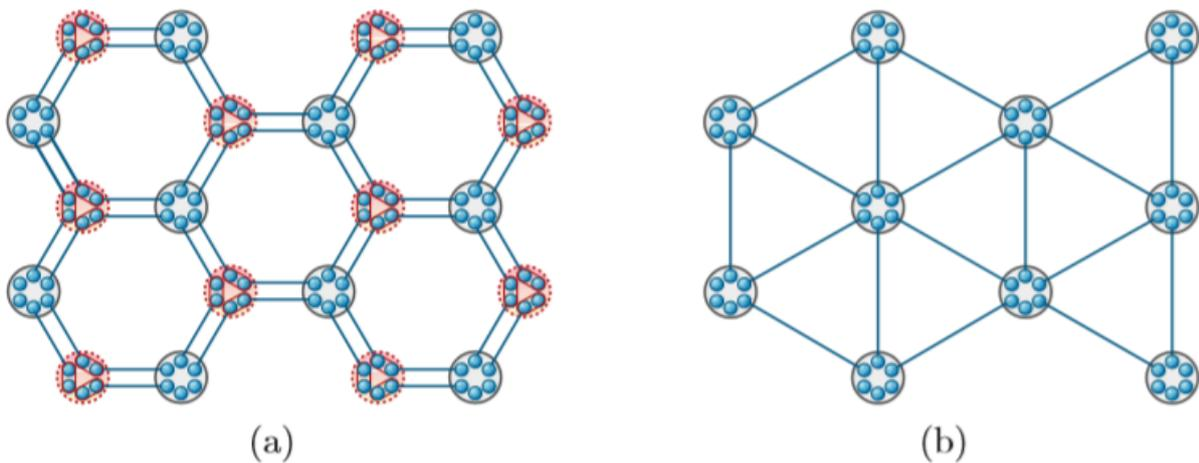
Figure 16: Transformation of Honeycomb Lattice to a Triangular Lattice ( which has a lower percolation threshold )
