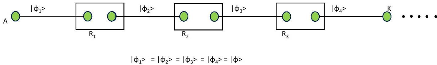
b) Multiple Repeater Configuration for analysing the exponential decay of concurrence and singlet conversion probability on employing entanglement swapping at the multiple repeaters.
