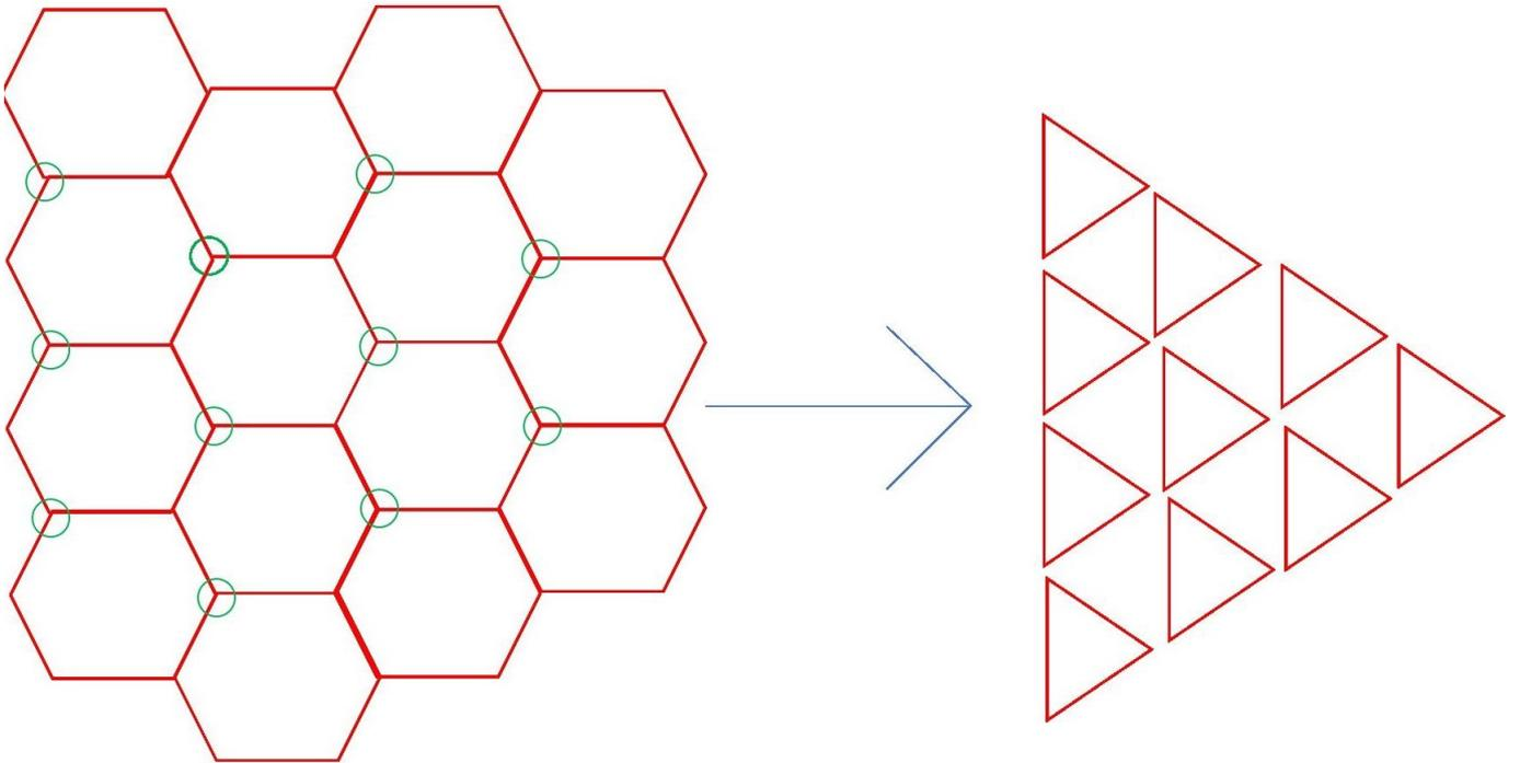
Figure 18: Conversion of the honeycomb lattice, consisting of partially entangled pure two-qubit states, to a triangular lattice, spanned by three-qubit partially entangled GHZ states
