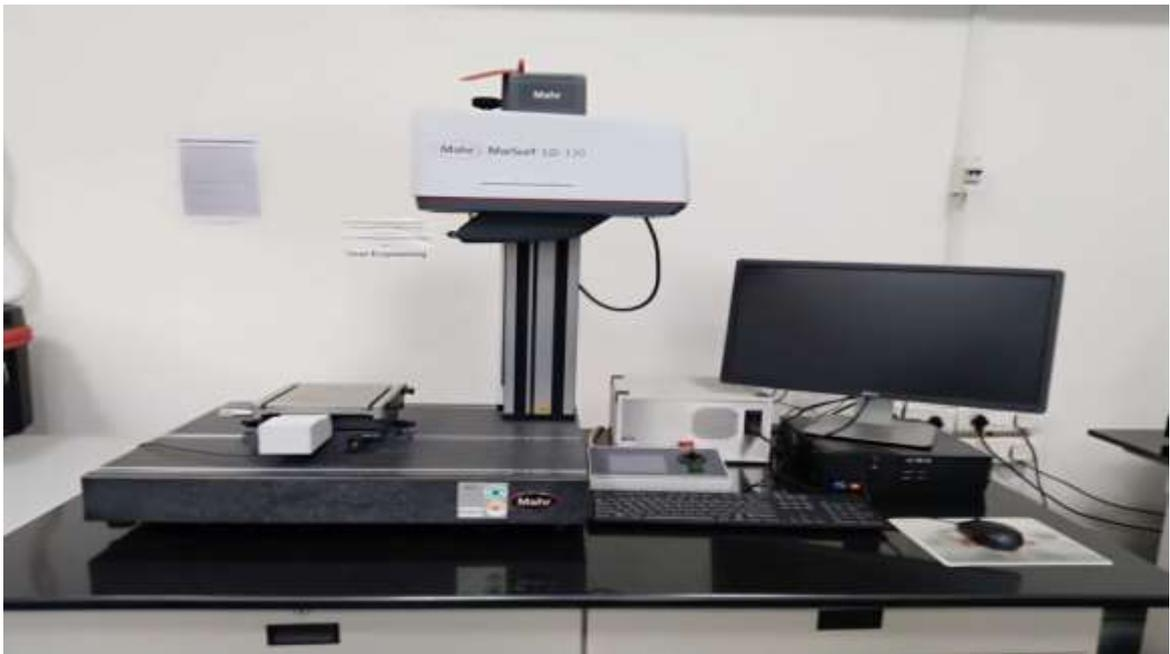
**Figure A1:** 3D Surface roughness-cum-contour tracing equipment.
