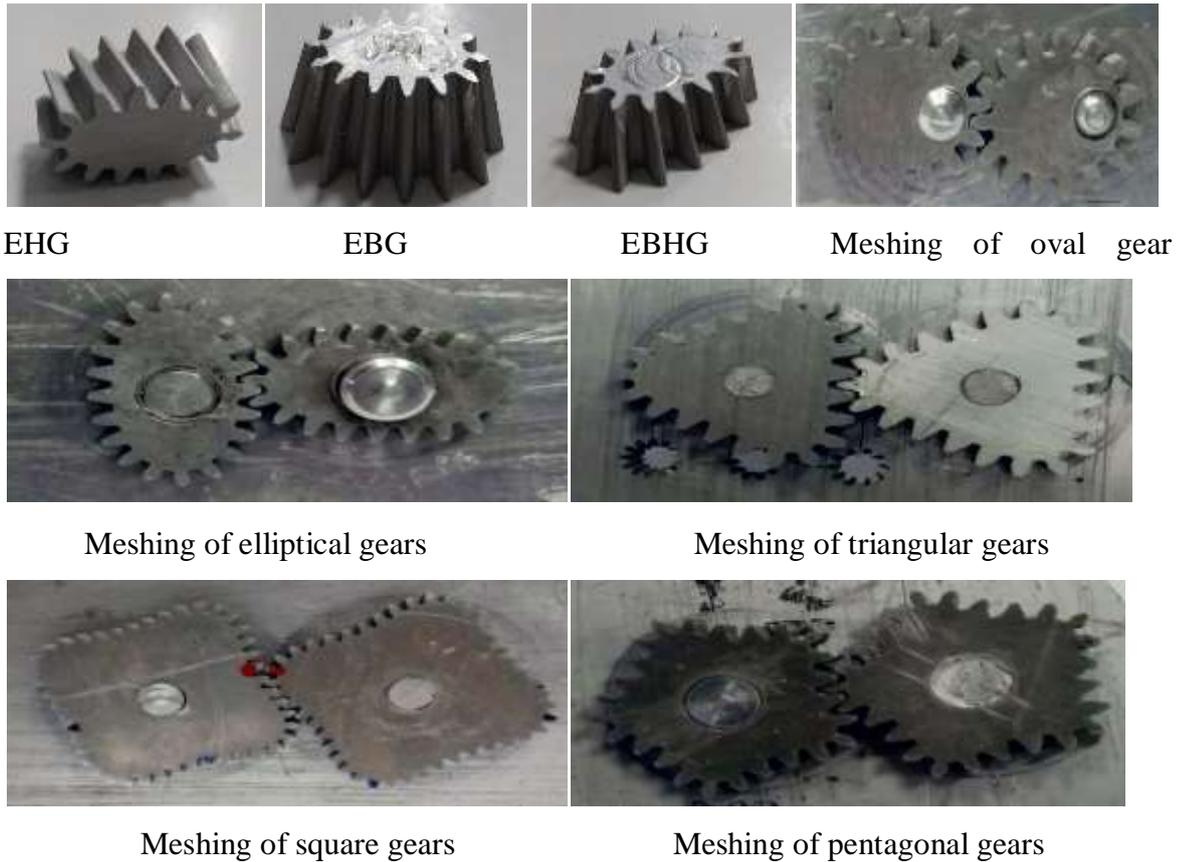
**Fig.4.2:** Macro-sized NCG of different types manufactured in Stage-1 experiment and their meshing arrangements.
