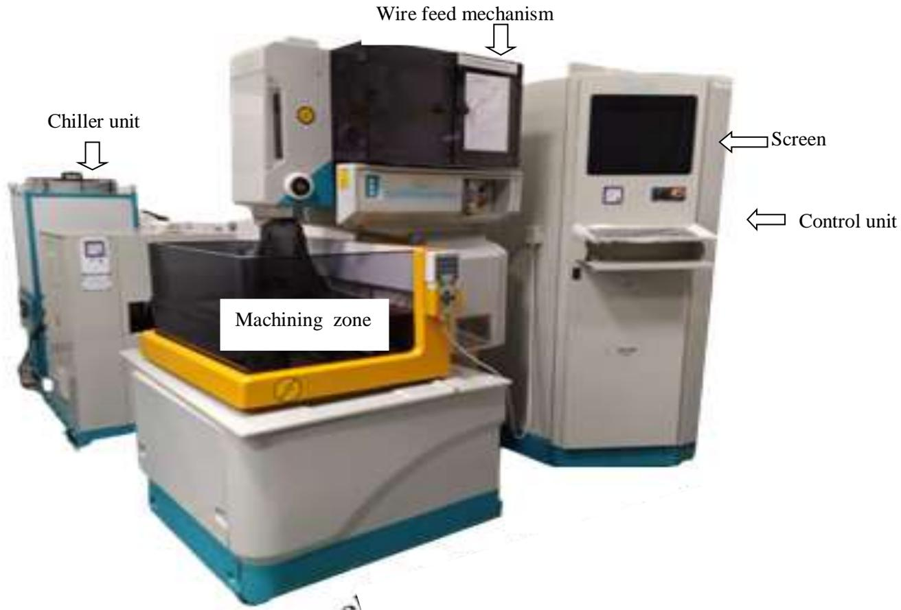
**Fig. 3.2:** Photograph of the *SprinCut-WINWSEM* used in the present work.
