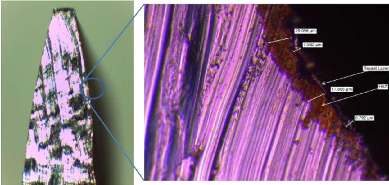
**Fig 4.10:** Heat affected zone (HAZ) and recast layer on tooth flank surface of the best quality EHG manufactured by WSEM process.
