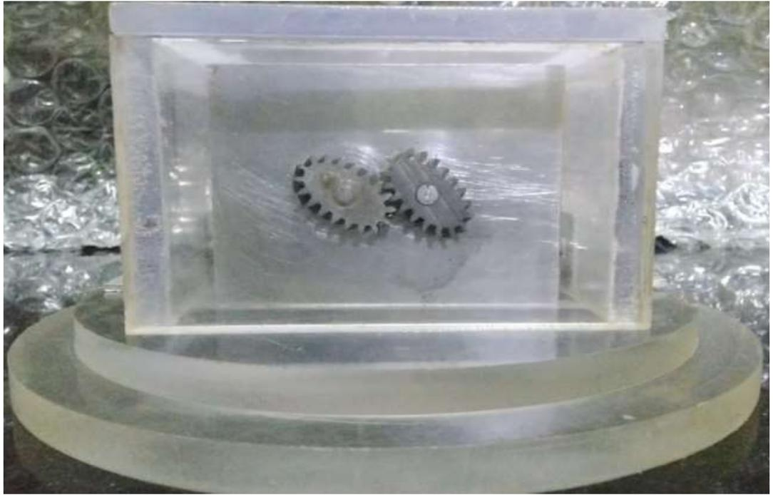
**Fig 4.11:** Apparatus for checking meshing of the EHG manufactured by WSEM process.
