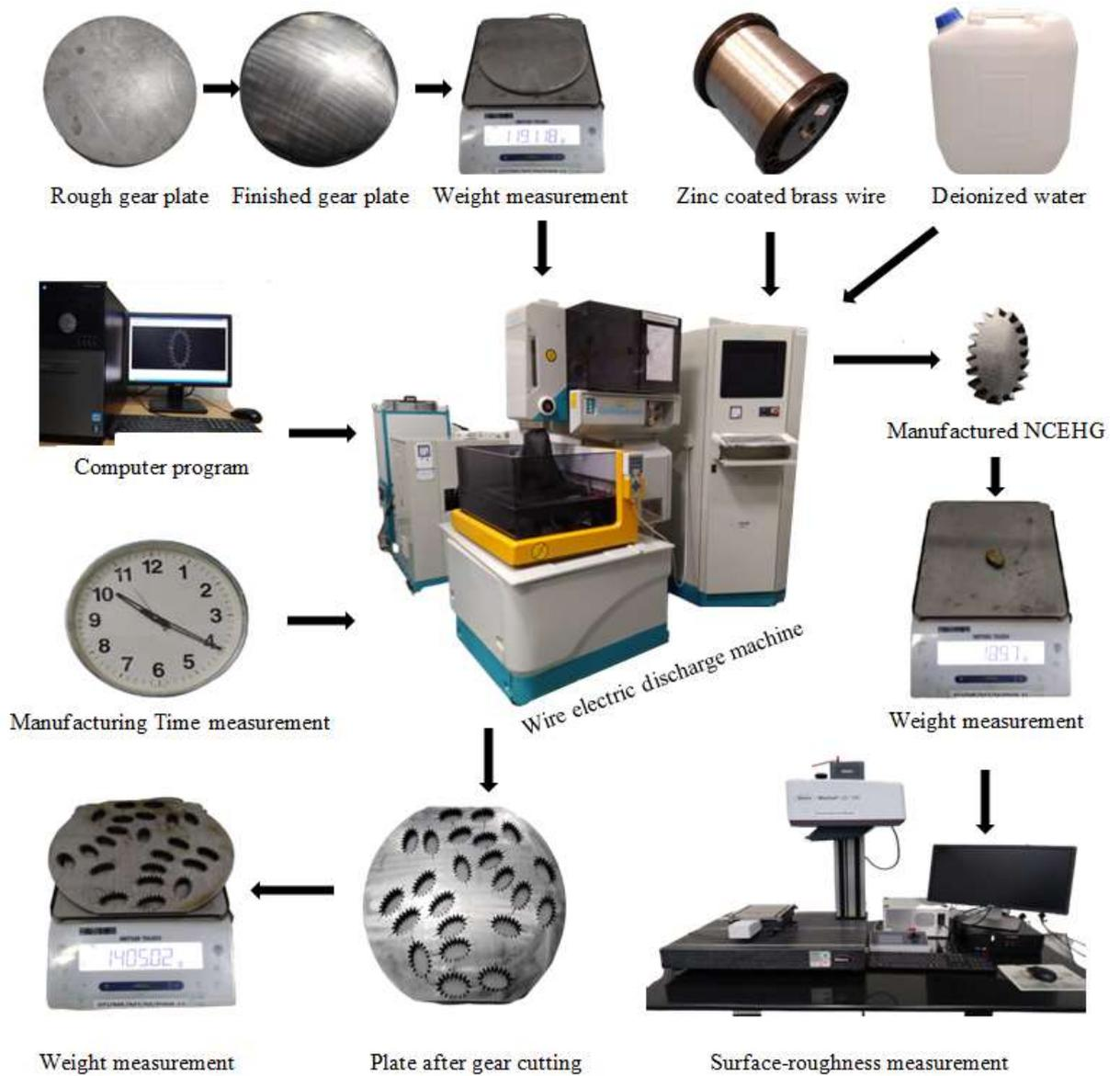
**Fig. 3.3:** Sequence of the different activities in manufacturing of EHG by WSEM process.
