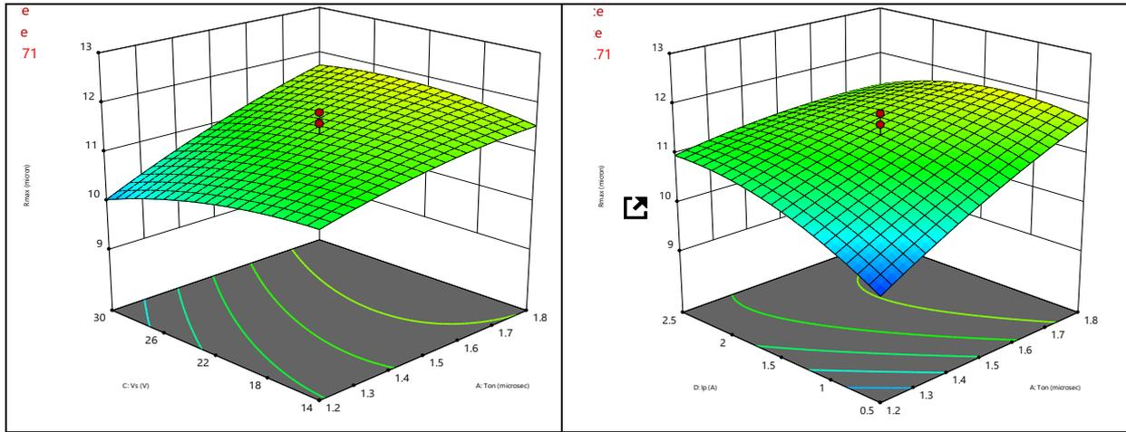
(a) For maximum roughness value of EHG flank surface ( $R_{max}$ )
