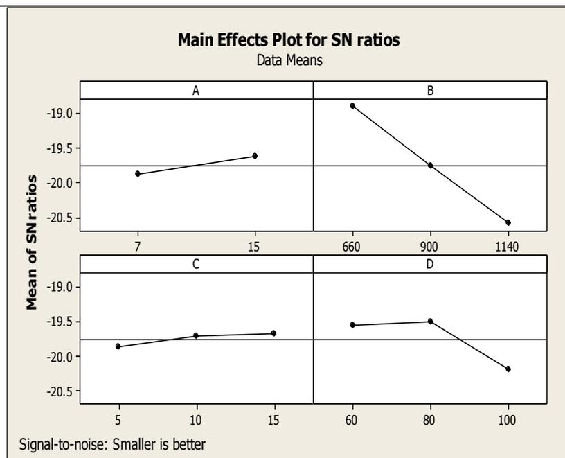
**(a) Maximum value of flank surface roughness ( $R_{max}$ )**
