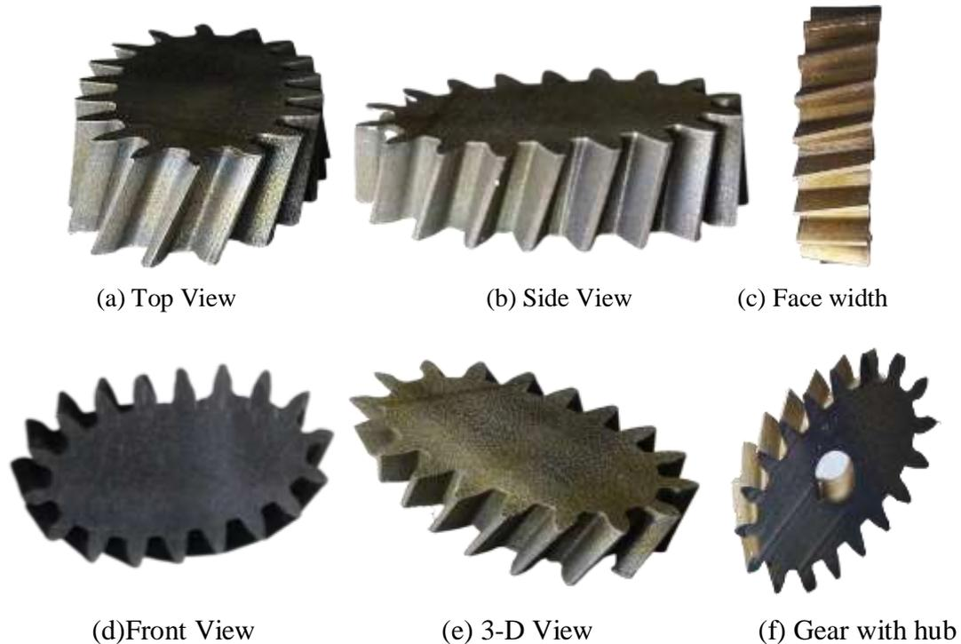
**Fig. 4.4:** Different views of the EHG manufactured using the GRA optimized WSEM process parameters.
