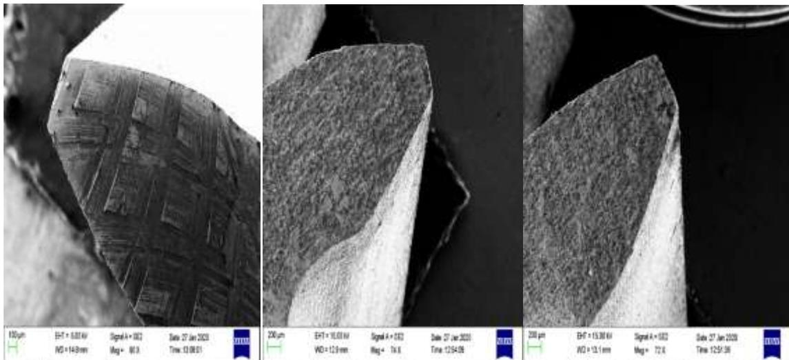
**Fig: 4.9:** Tooth profile of the best quality EHG manufactured by WSEM process.
