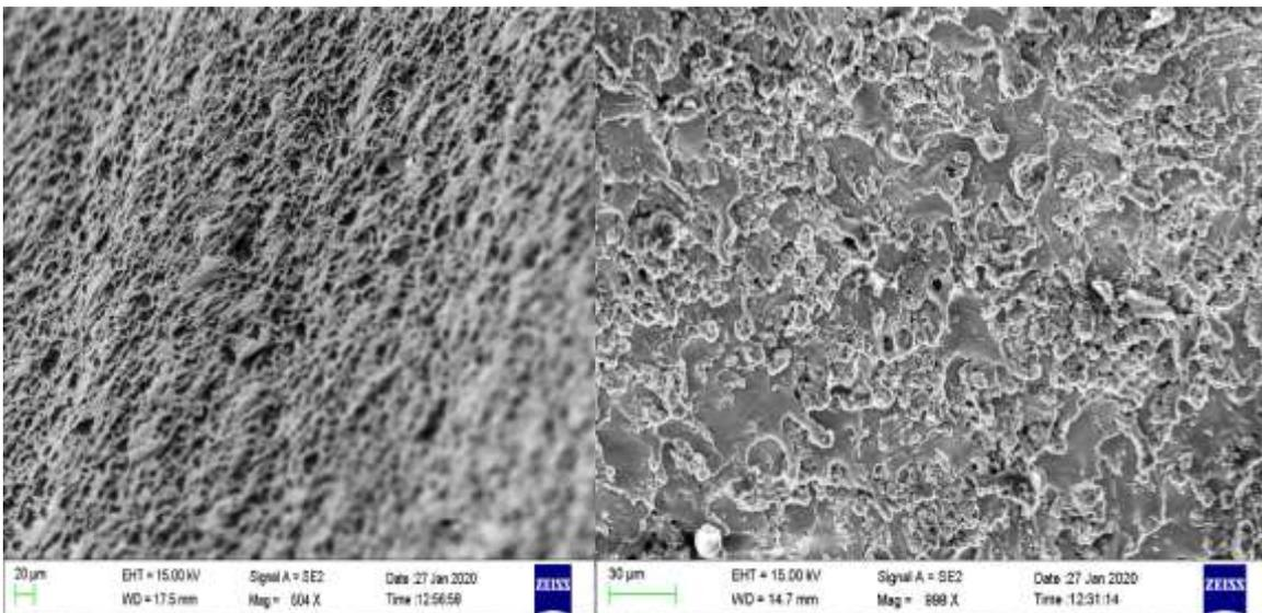
**Fig. 4.8:** Topography of flank surface of the best quality EHG manufactured by WSEM.
