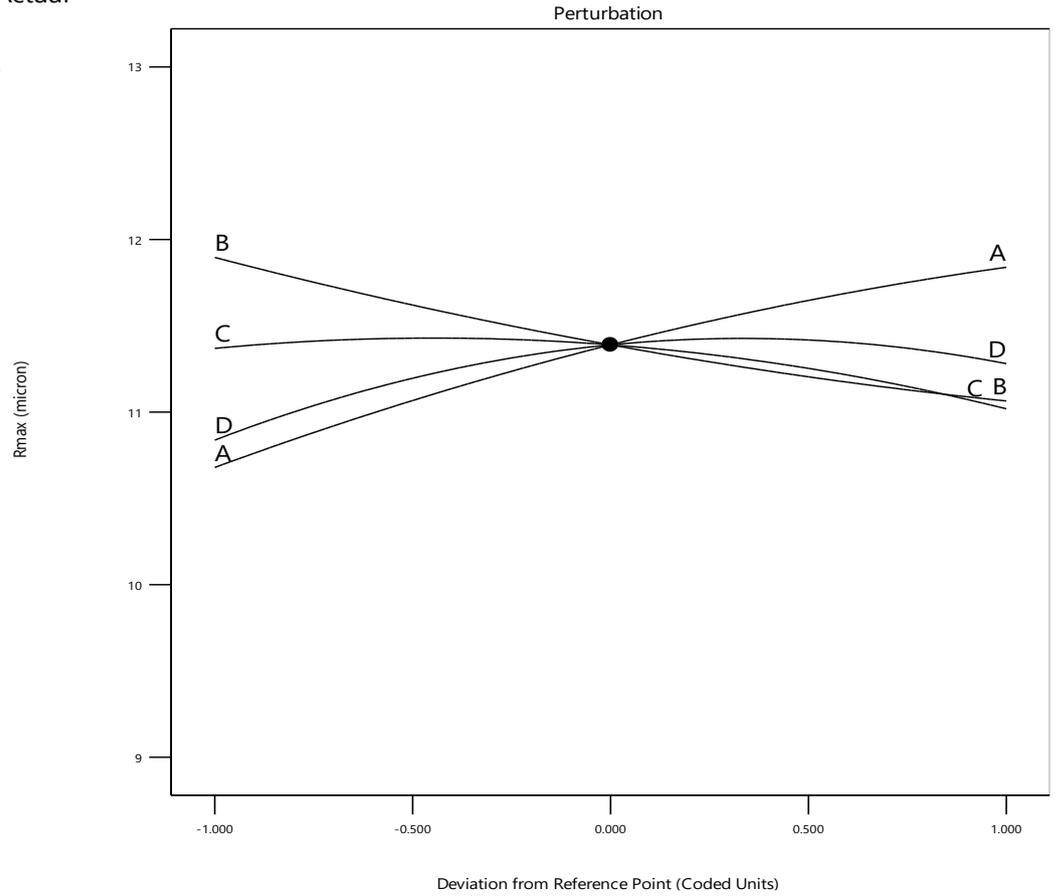
**(a) Maximum roughness value of EHG flank surface ( $R_{max}$ )**
