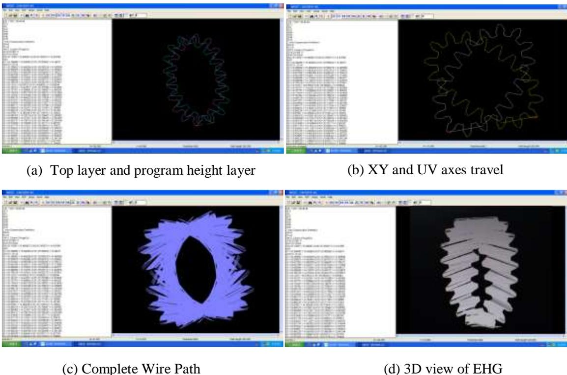
**Fig. 3.1:** Different views of wire path programmed by the ELCAM software.
