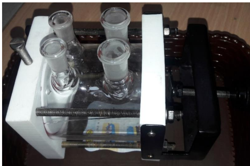
Figure 7: CHI604E Potentiodynamic Polarizing Electrochemical Corrosion Setup
