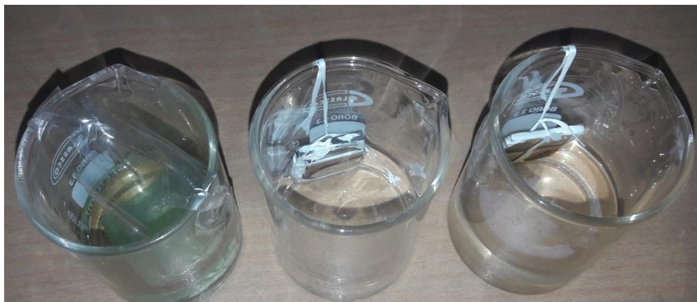
Figure 5b: FeCoNiCrVZr 0 HEA samples in 3M of HCl, NaCl and NaOH kept to stabilize for 20 days
