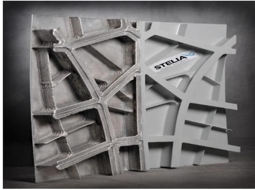
**Figure 1.7 Aluminium fuselage of aeroplane made by SLM [3]**
