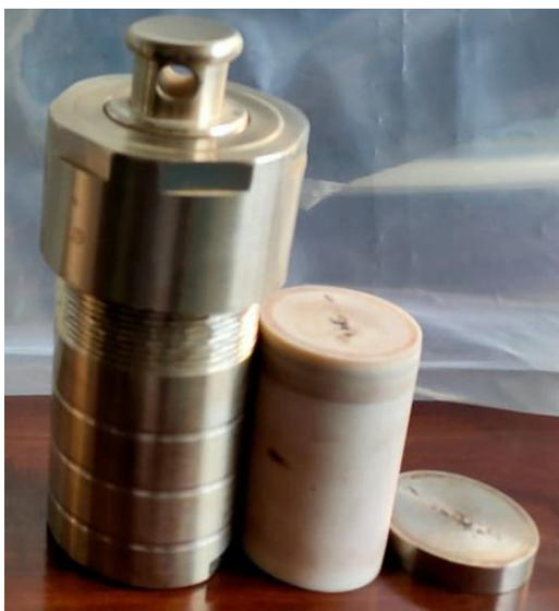
**Figure 2.4.** *Stainless steel Teflon lined autoclave used in this thesis work.*
