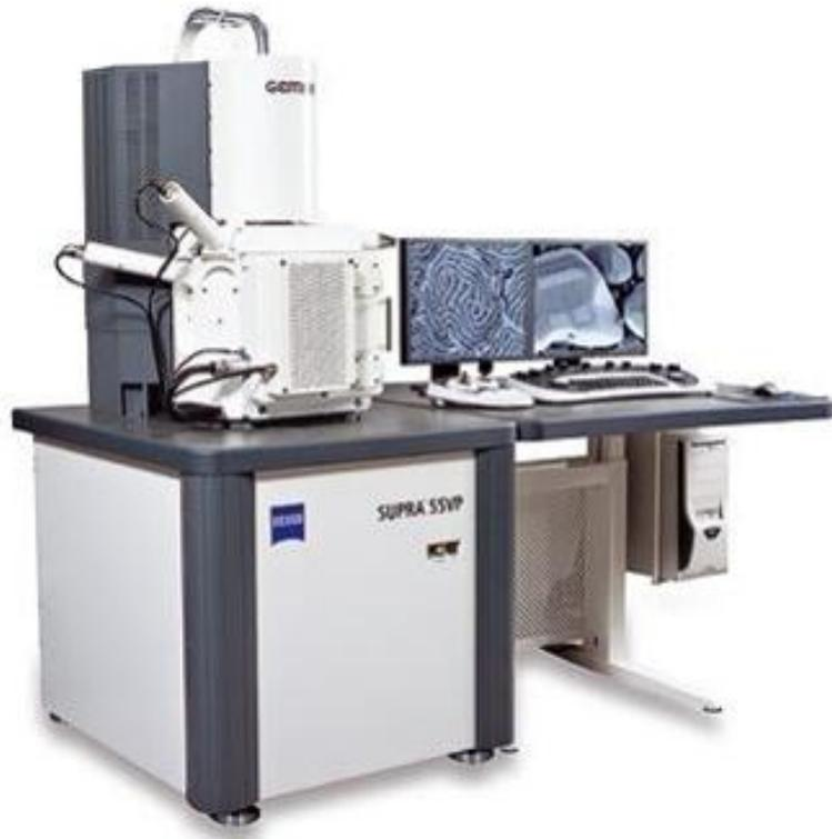
*Figure 2.13. Image of the FESEM/EDX system, ZEISS Supra<sup>55</sup>.*
