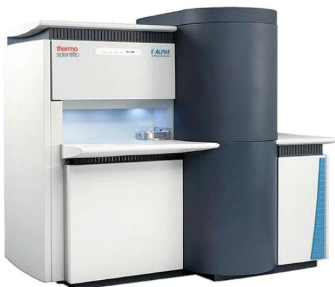
*Figure 2.18.* Image of the XPS system used in the present thesis work.
