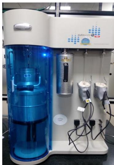
*Figure 2.22. Image of the Autosorb iQ2, used in the present thesis work for BET surface area analysis.*
