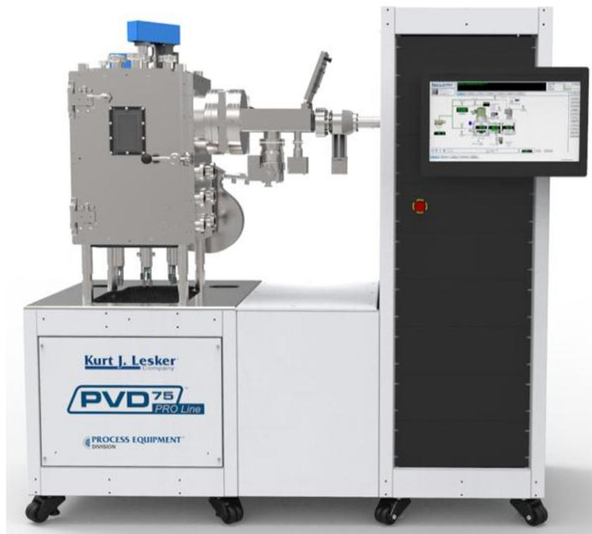
**Figure 2.8.** The system used to grow seed layer and metal electrodes in this work.
