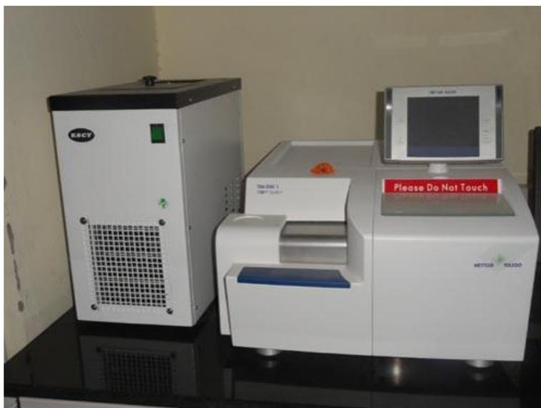
*Figure 2.20. Image of the Mettler Toledo Thermal Analyzer used in this thesis work.*
