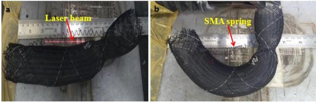
**Fig. 3.29:** Soft mesh structure bending during laser actuation
