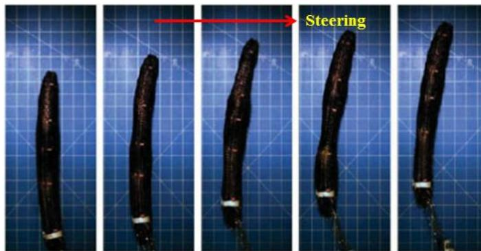
**Fig. 2.4:** SMA spring based meshworm robot [29]
