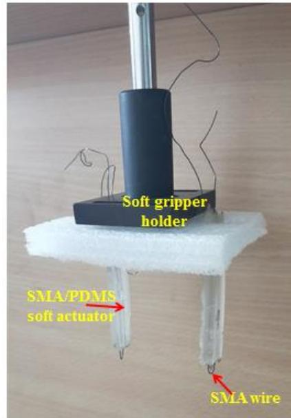
**Fig. 8.4:** Prototype of SMA wire based soft robotic gripper
