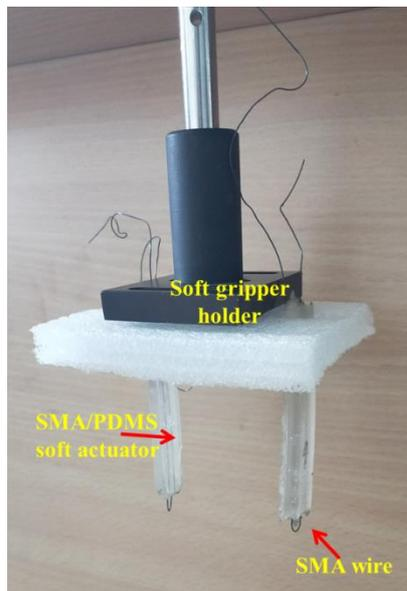
**Fig. 6.13:** SMA/PDMS based soft robotic gripper
