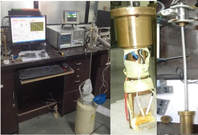
**Figure-2.6 Schematic diagram Low Temperature Dielectric Experimental Setup.**
