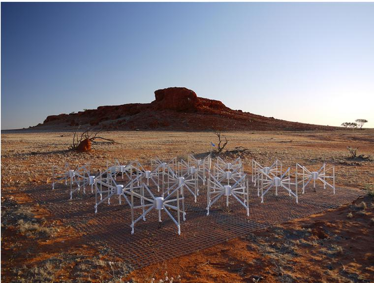
Figure 2.1: Array of dipole antennas- MWA [8].
