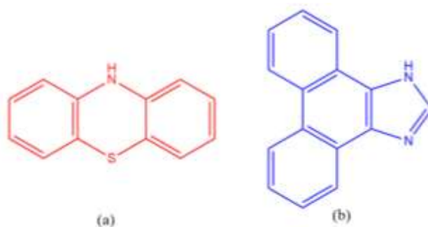
Figure 3: Chemical structure of (a) Phenothiazine and (b) Phenanthroimidazole molecule
