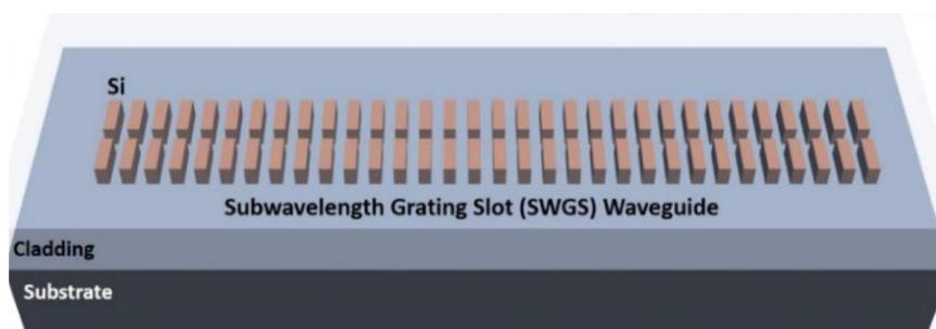
**Figure 2.9** 3D structure of a subwavelength grating slot waveguide. The period, silicon rib width and slot width are kept at 200 nm, 300 nm, and 100 nm. [82]
