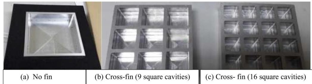
**Fig. 1.9** Square cross finned heat sink considered by Leong et al. [150]
