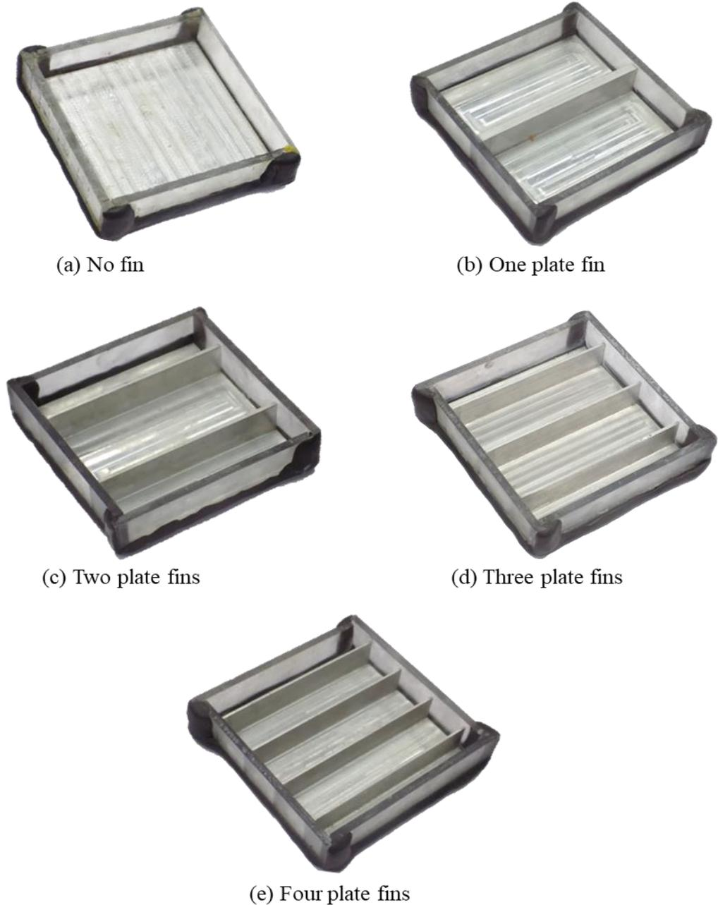
**Fig. 4.30** Photographs of various heat sinks used in this investigation
