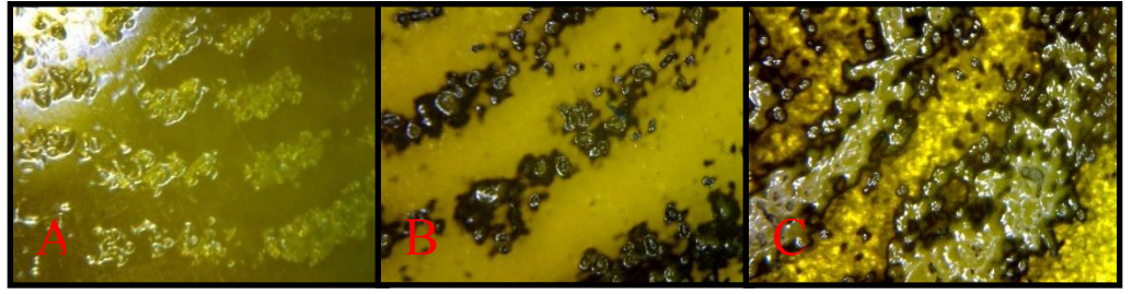
Figure 4.8 Image of ripple ring formed during direct texturing of polyimide at (A) 355nm (B) 532nm(C) 1064nm
