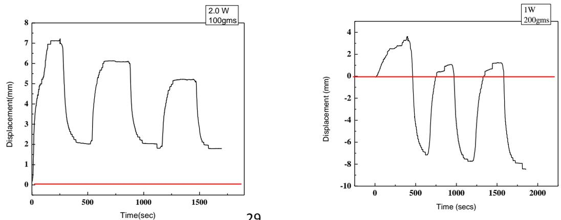
Figure 23: Displacement-Time relationship at varying load and power conditions
