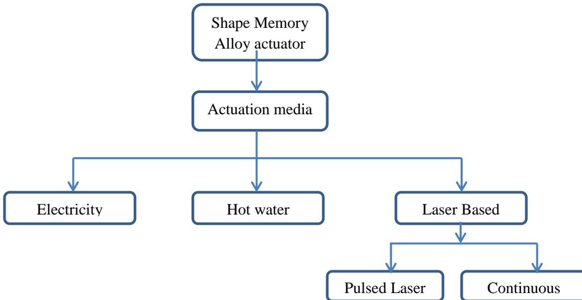
**Figure 5 Block diagram for different actuation media**
