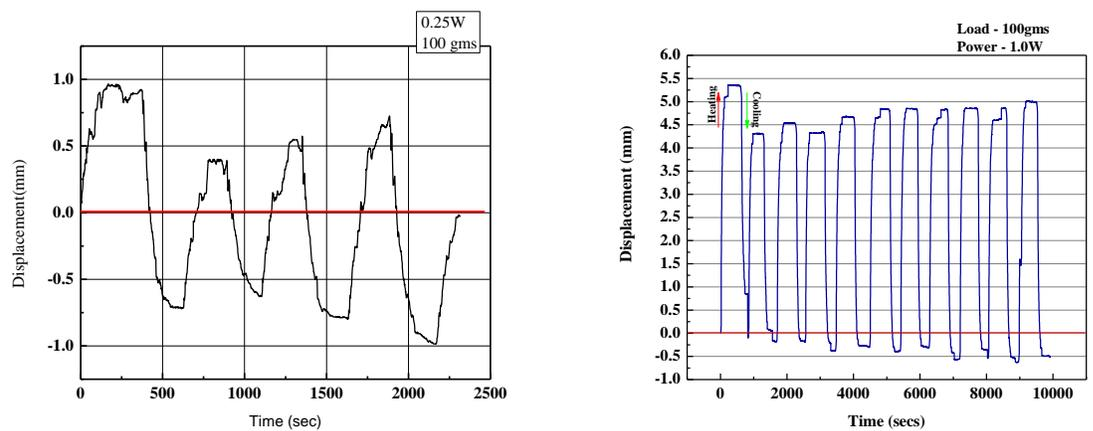
Figure 22: Displacement-Time relationship at 0.25 W and 1.0W
