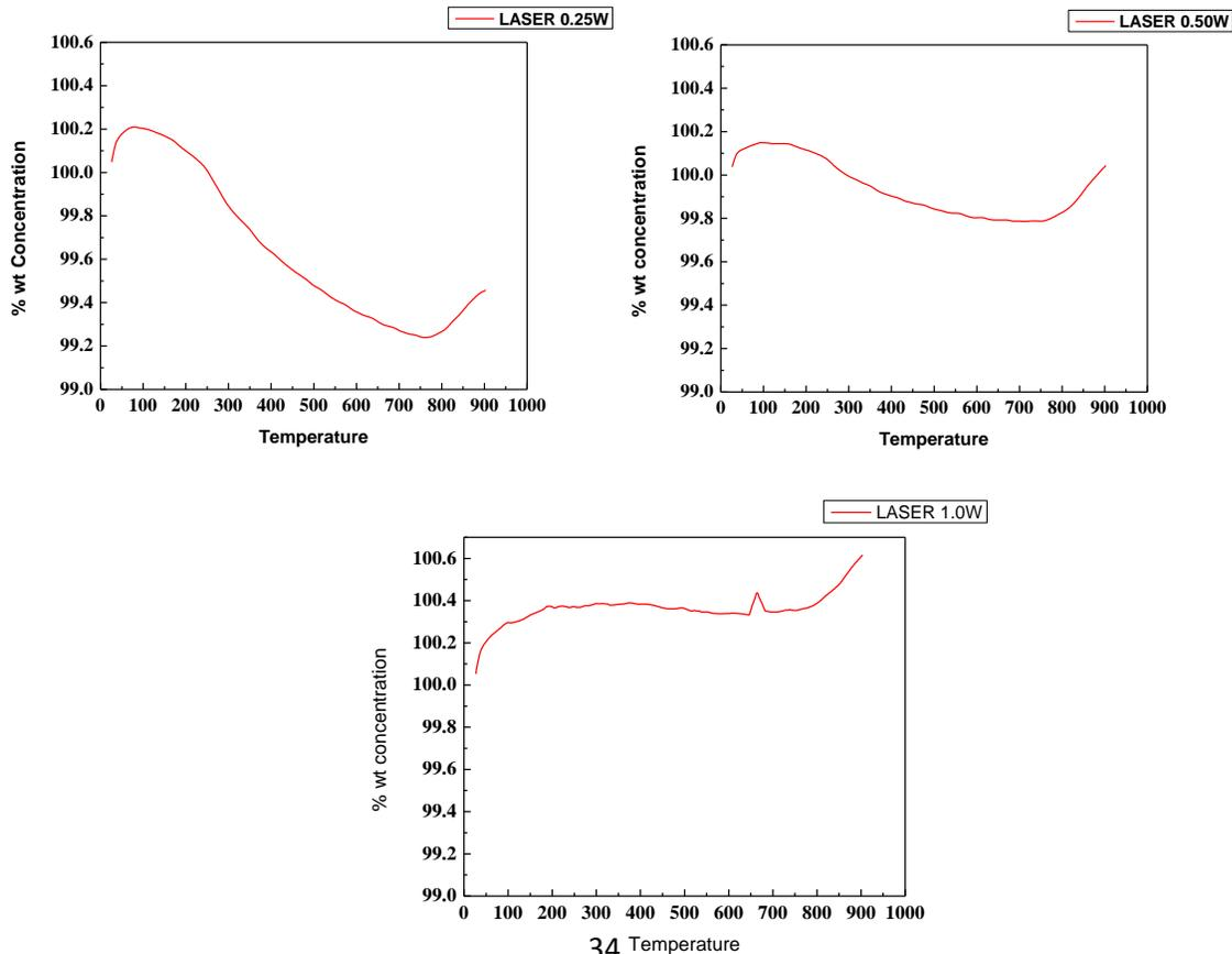
Figure 28: TGA analysis performed for springs undergoes heating at different laser powers (a) 0.25W, (b) 0.50W, (c) 1.0W
