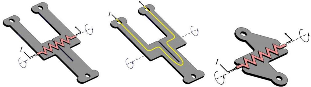
**Figure 7: Electrical circuit representation of the models. (a) Y-type: Ni–Cr heating, (b) Y-type: Joule heating and (c) Z-type: Ni–Cr heating(Paik 2010)**
