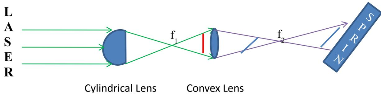
Figure 18: Schematic showing lens arrangement with their focal points
