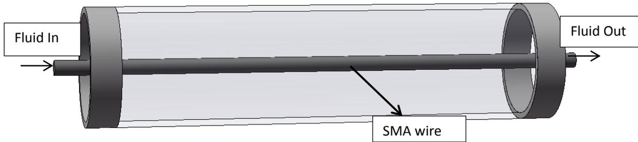
Figure 8: Wet SMA actuator design concept (Pierce 2011)
