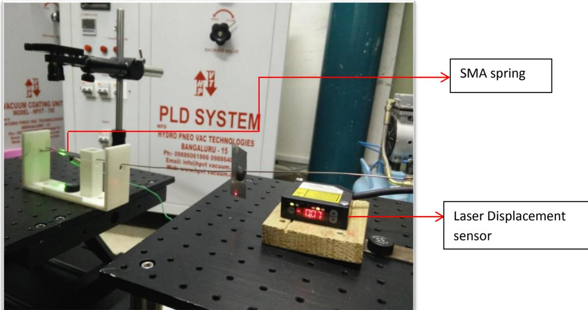
**Figure 15: Displacement calculation using LDS and flapper arrangement**
