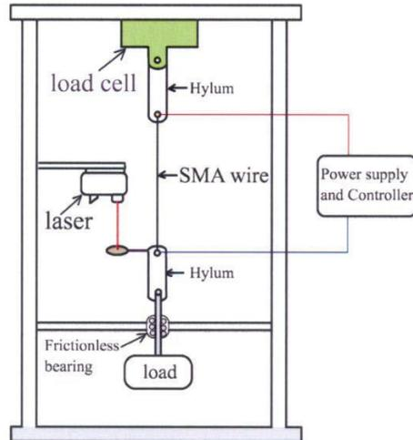
**Figure 6: Experimental setup consisting of SMA wire (Saikrishna (2009))**
