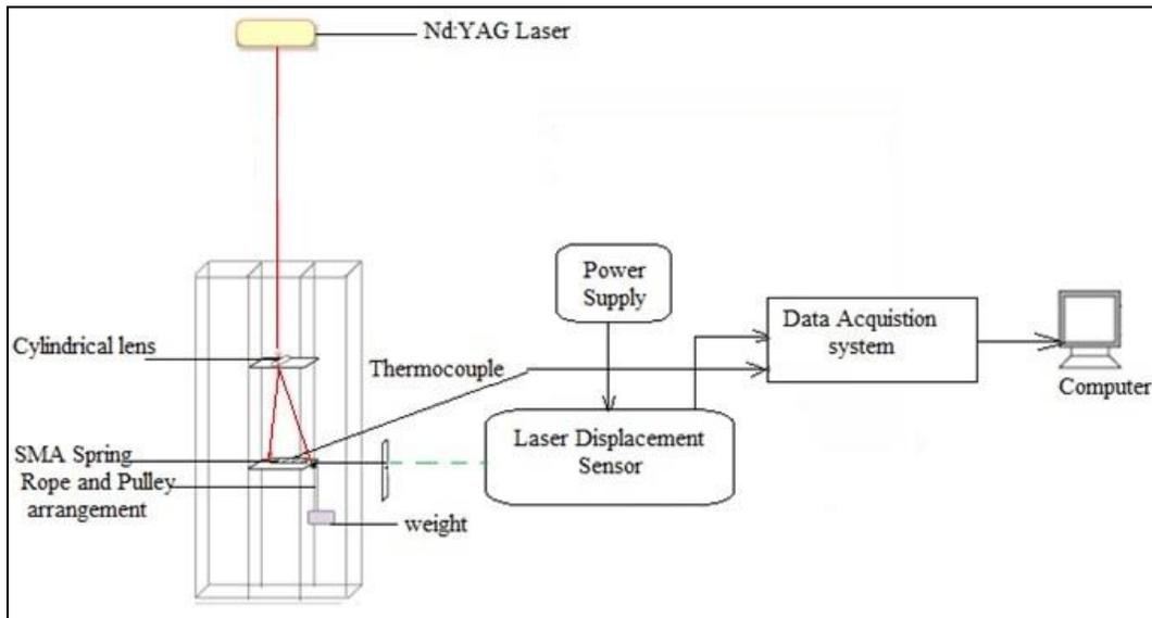
**Figure 13: Schematic for laser based actuation setup**
