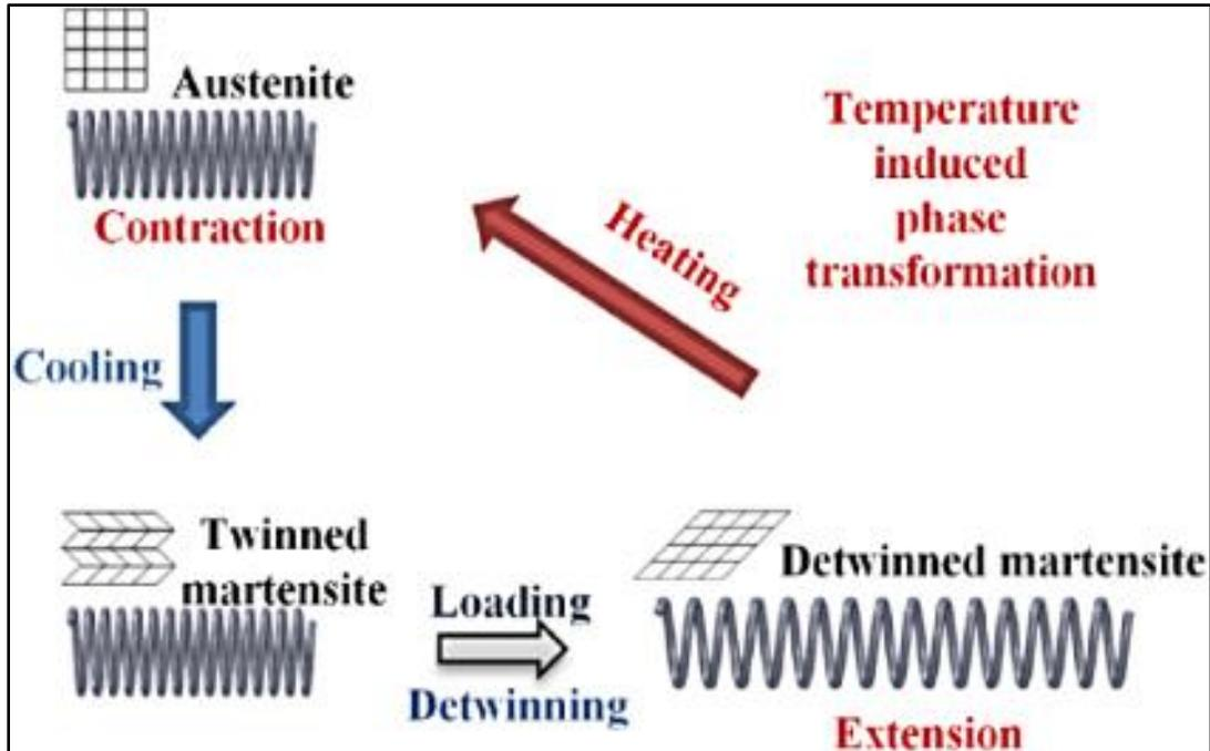
Figure 1 Crystalline arrangement of SMA in different phases (Wikipedia)
