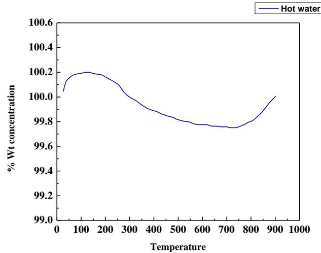
**Figure 36: TGA analysis for Hot water actuated spring**
