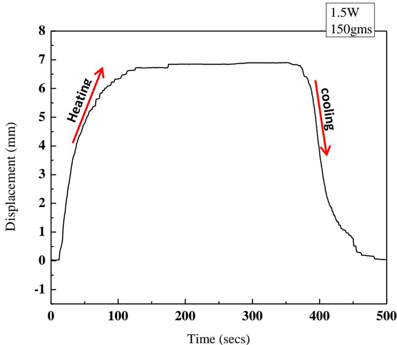
Figure 24: Single Heating-cooling cycle
