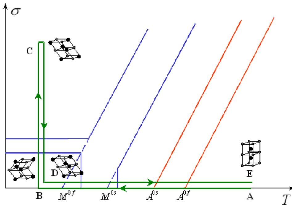
Figure 3: Schematic representation of the thermomechanical loading path demonstrating the shape memory effect in an SMA (Smart lab, Texas)
