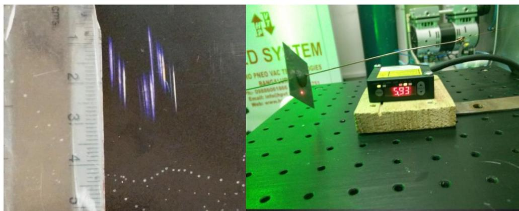
Above Figure shows the line obtained with quartz tube captured in a photographic sheet in normal view with a centimeter scale kept parallel to it as reference.
