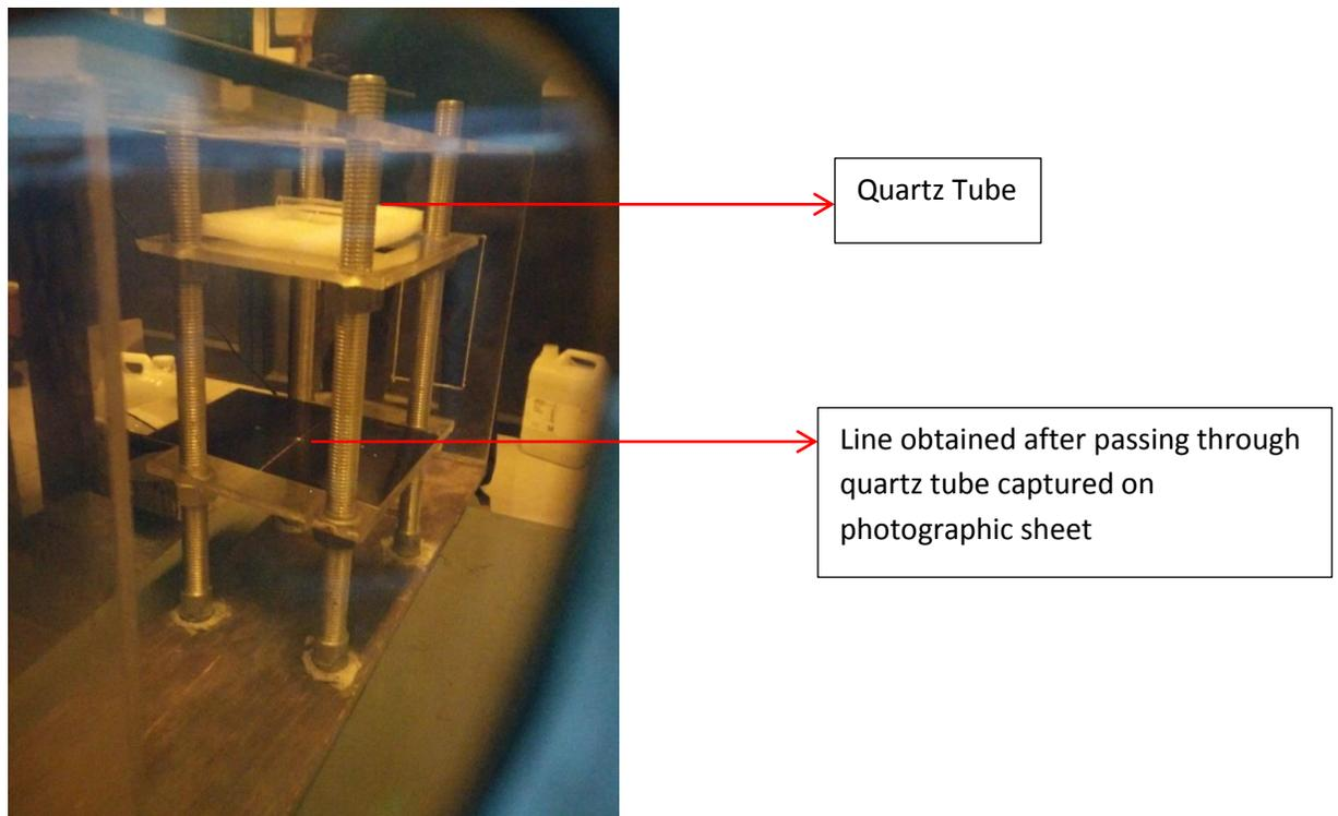
**Figure 14: Experimental setup using quartz tubes**
