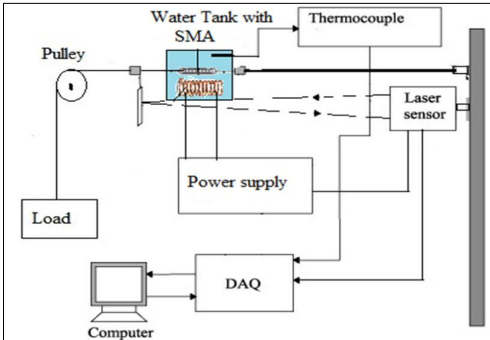
**Figure 19: Schematic for hot water actuation setup**
