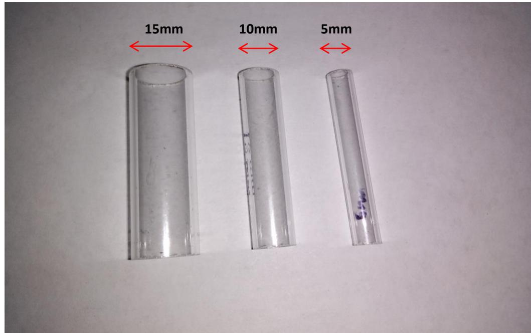
**Figure 12 Quartz tubes used with varying diameters**
