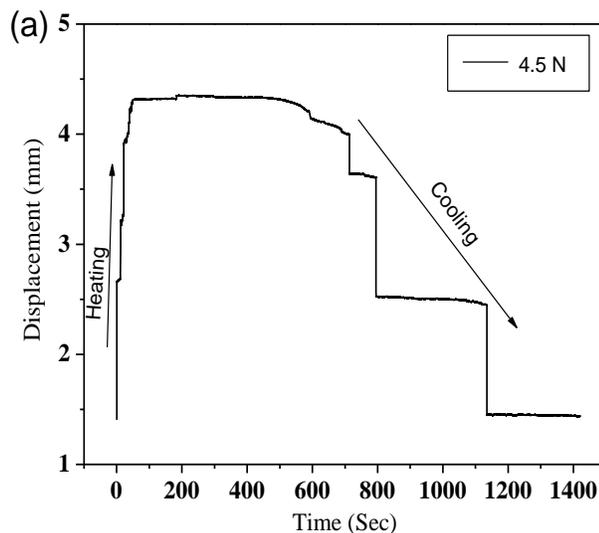
Figure 33: Displacement Vs. Time relation for Hot water actuation
