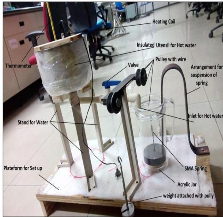
**Figure 20: Experimental setup for Hot water actuation method**
