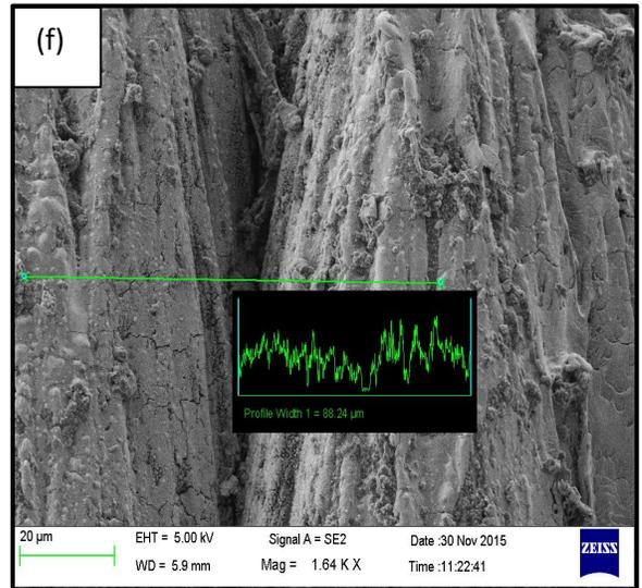
**Figure 26: SEM images at different powers (a) Sample cut of 10mm, (b) Original Sample, (c) 0.25W, (d) 1.0W, (e) 2W, (f)Depth created due to high power**
