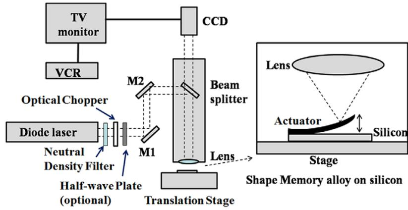
Figure 9: Schematic of the optical-microscope-focused laser beam system (Hu 2012)
