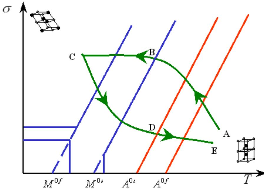
Figure 4: Schematic of a thermomechanical loading path demonstrating pseudoelastic behavior of SMAs. (Smartlab, Texas)
