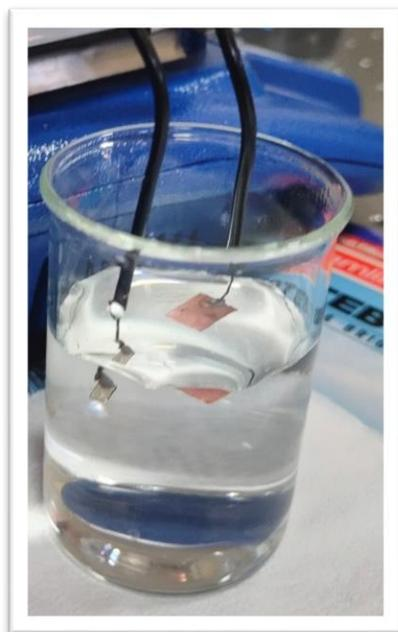
**Figure 2.6:** Hydrogenation *via* metal-acid contact method under a mild electric field.
