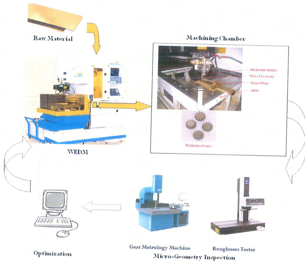
Fig. 2: Tasks and equipments used in experimental investigations on miniature gear manufacturing by WEDM.
