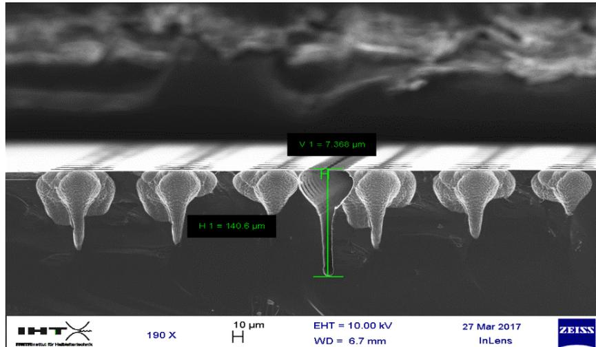
Figure 31. SEM image of the device after TEST 1.
