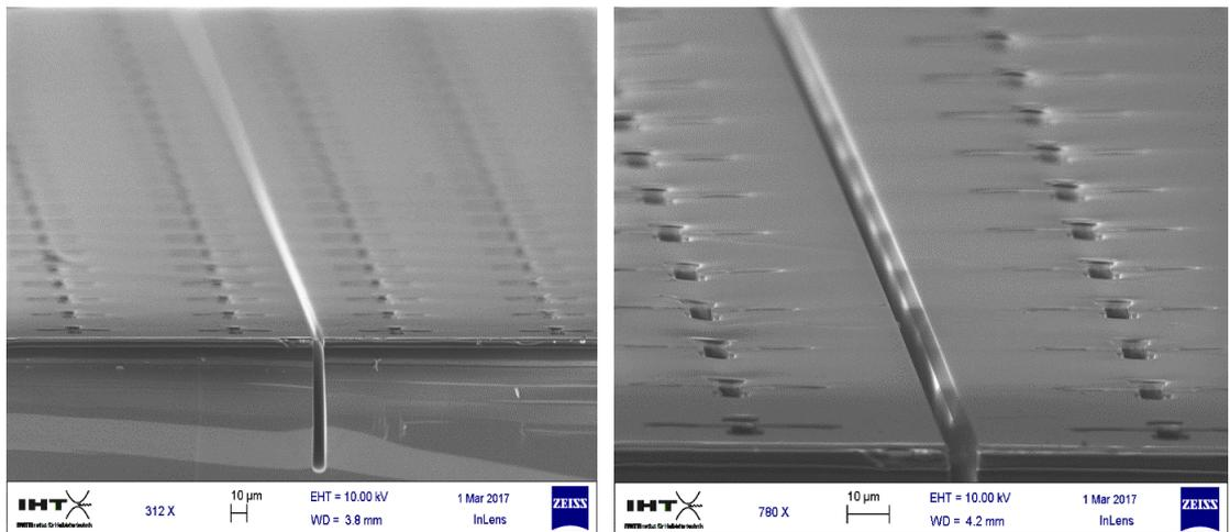
Figure 21. SEM image of the Surface of the device after Bosch etching for 30 minutes
