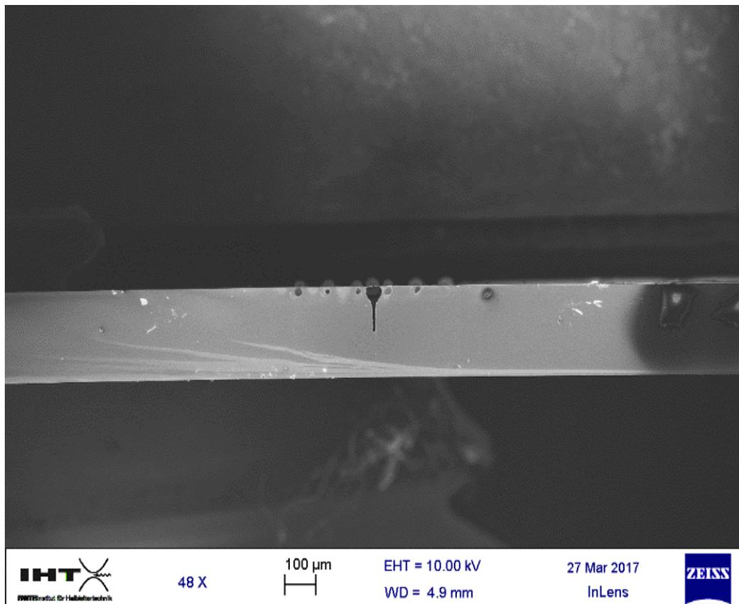
*Figure 33. SEM image of the strained device after Test 2*
