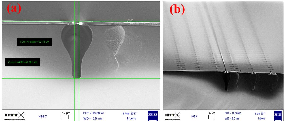
Figure 24. (a) & (b) Etching depth of 82.33 micron after 1 time Bosch + 2 times Isotropic etch.
