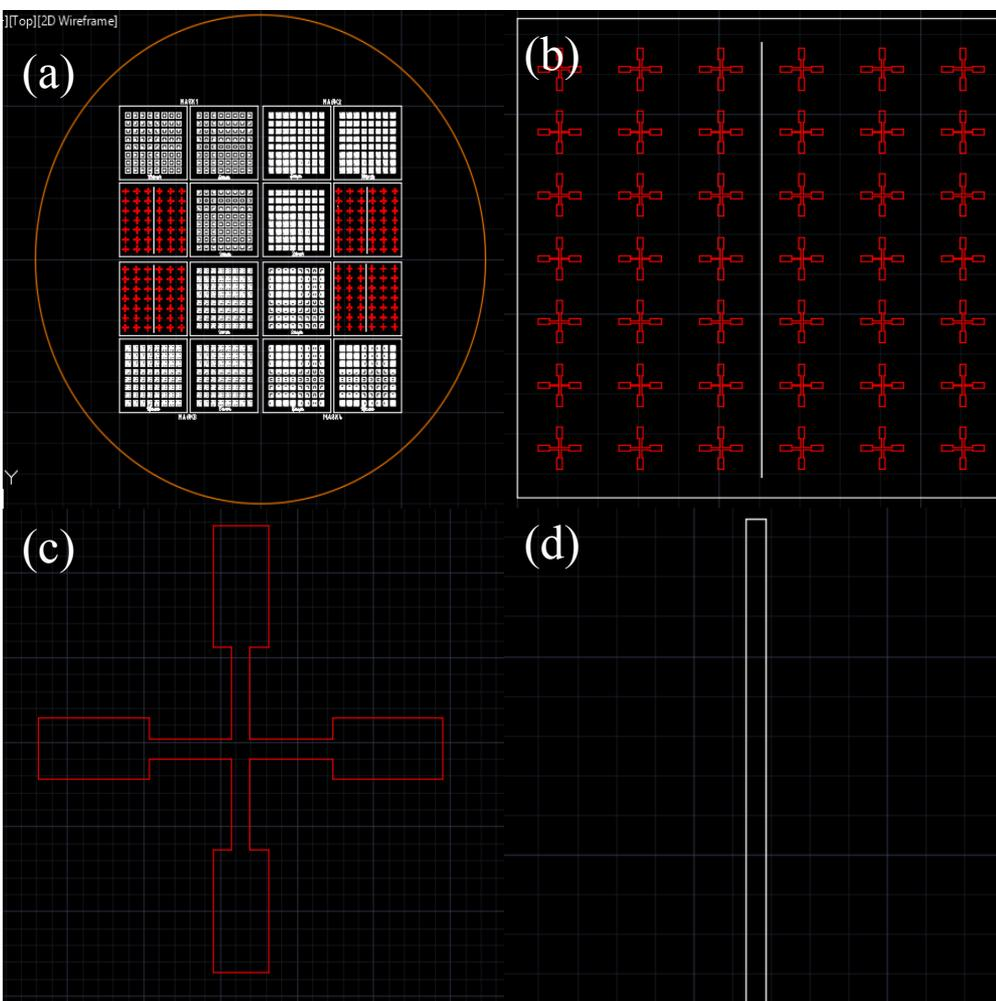
Figure 8. . a) Overall Mask view. b) Trench line in the middle with Marker structure on either side. c) A Marker structure in a large view. d) Trench line in large view
