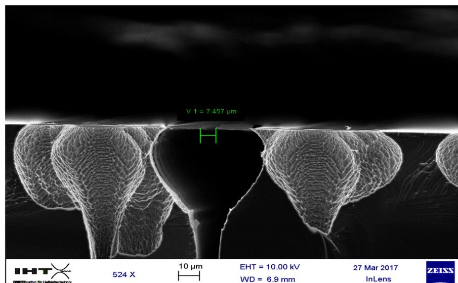
Figure 35. Width of opening of trench after strain Test 3
