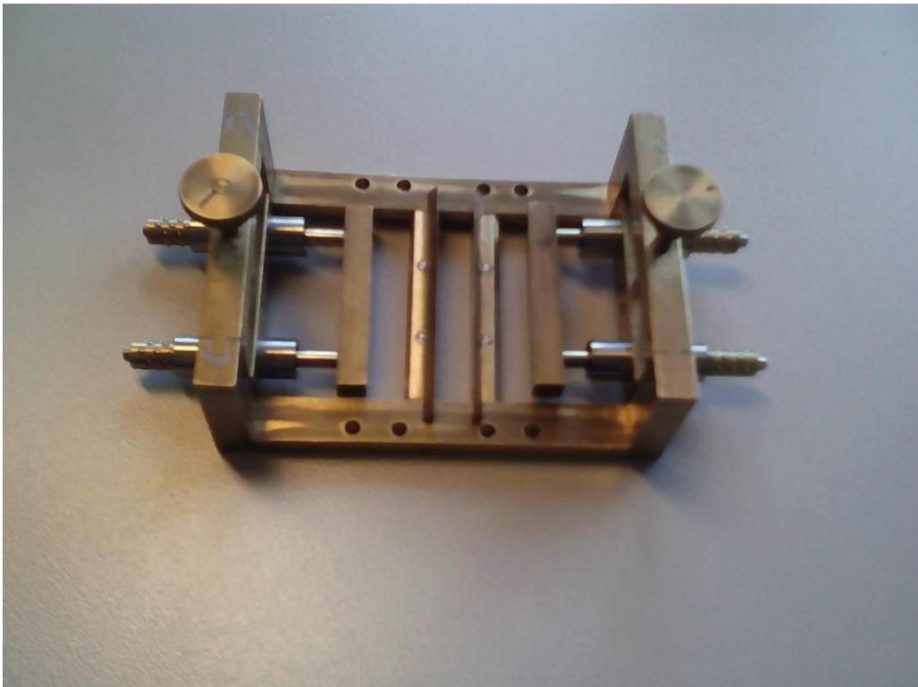
*Figure 28. A Setup with top & side screw to Create Strain in Sheets/Wafer type material.*
