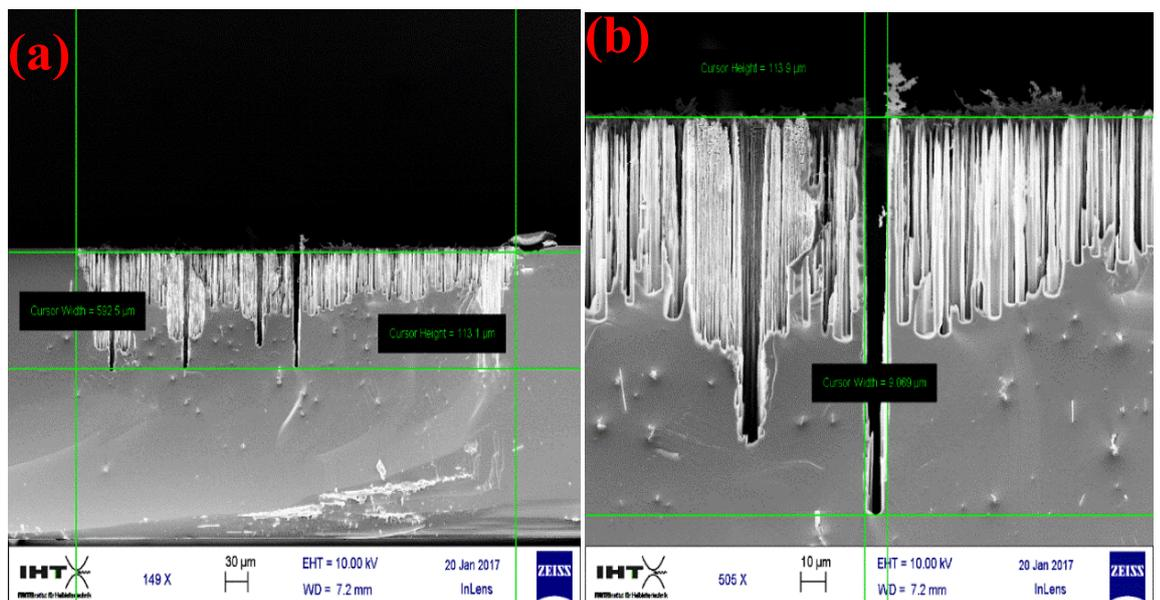
Figure 17. (a) & (b) showing the SEM image of sample with Method 1 after final etching.
