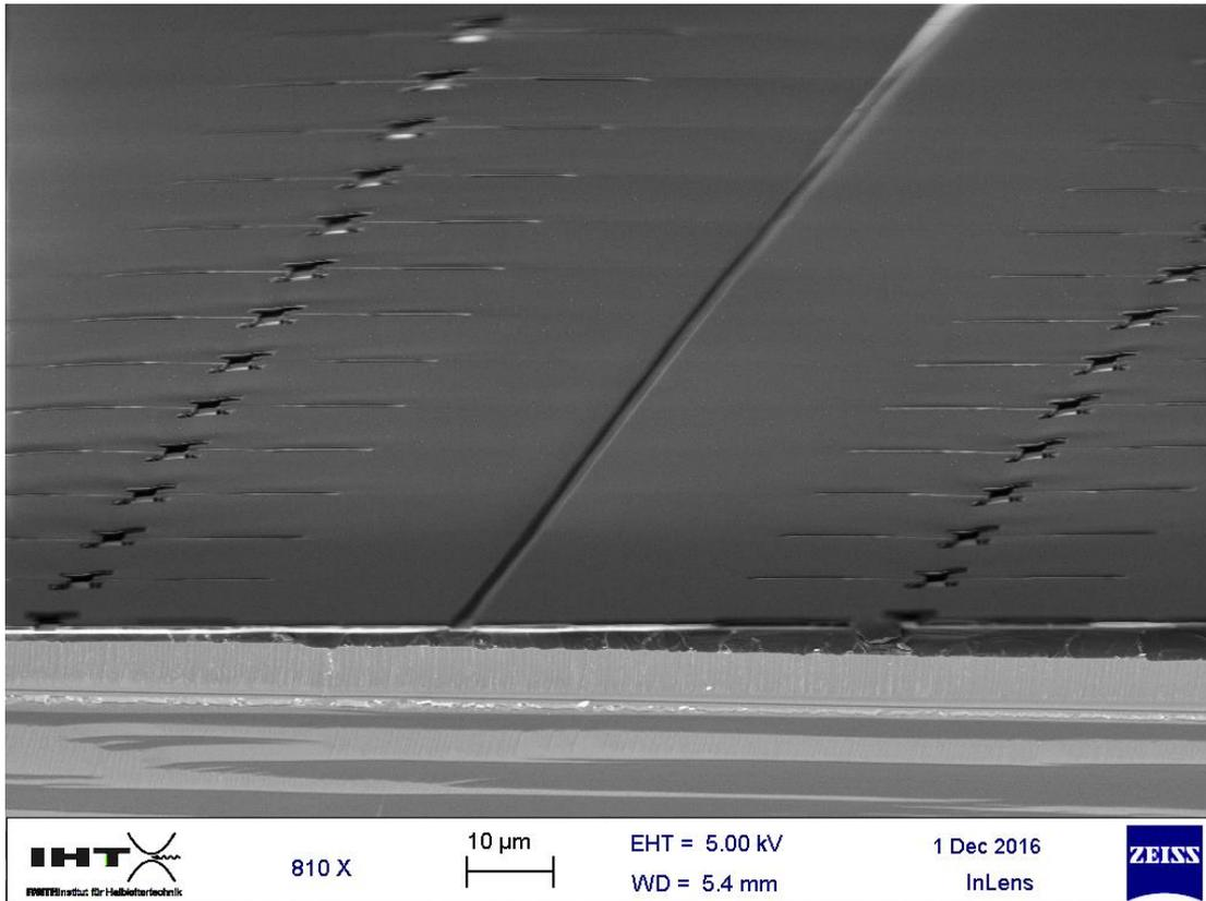
Figure 10. SEM image of the sample after optical lithography and development
