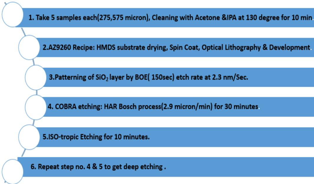
Figure 23. Final Process flow for the device fabrication.
