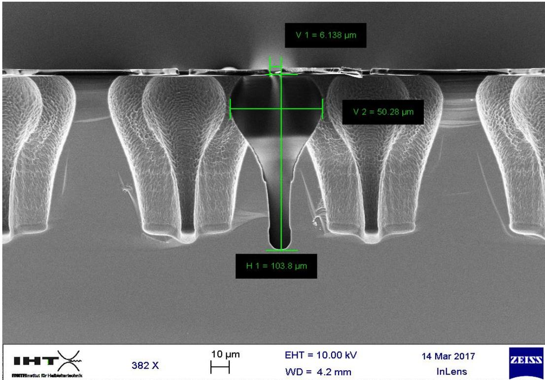
Figure 25. SEM image of etching profile after 30min Bosch + 10min Isotropic etch
