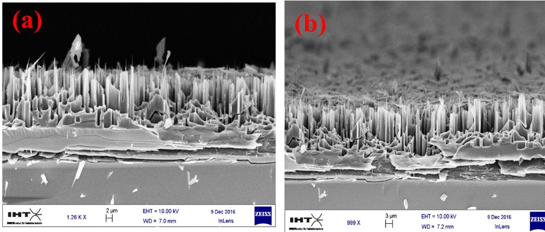
Figure 12. (a) & (b) Showing the sample's surface after Cryogenic etch for 50 minutes
