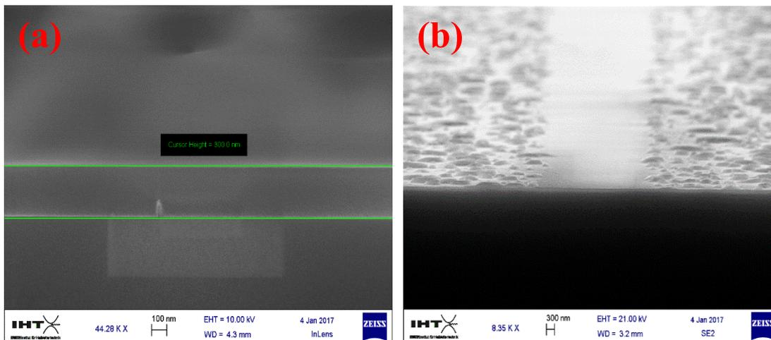
Figure 14. (a) Thickness of alumina layer deposited. (b) Instability of PR due to BOE
