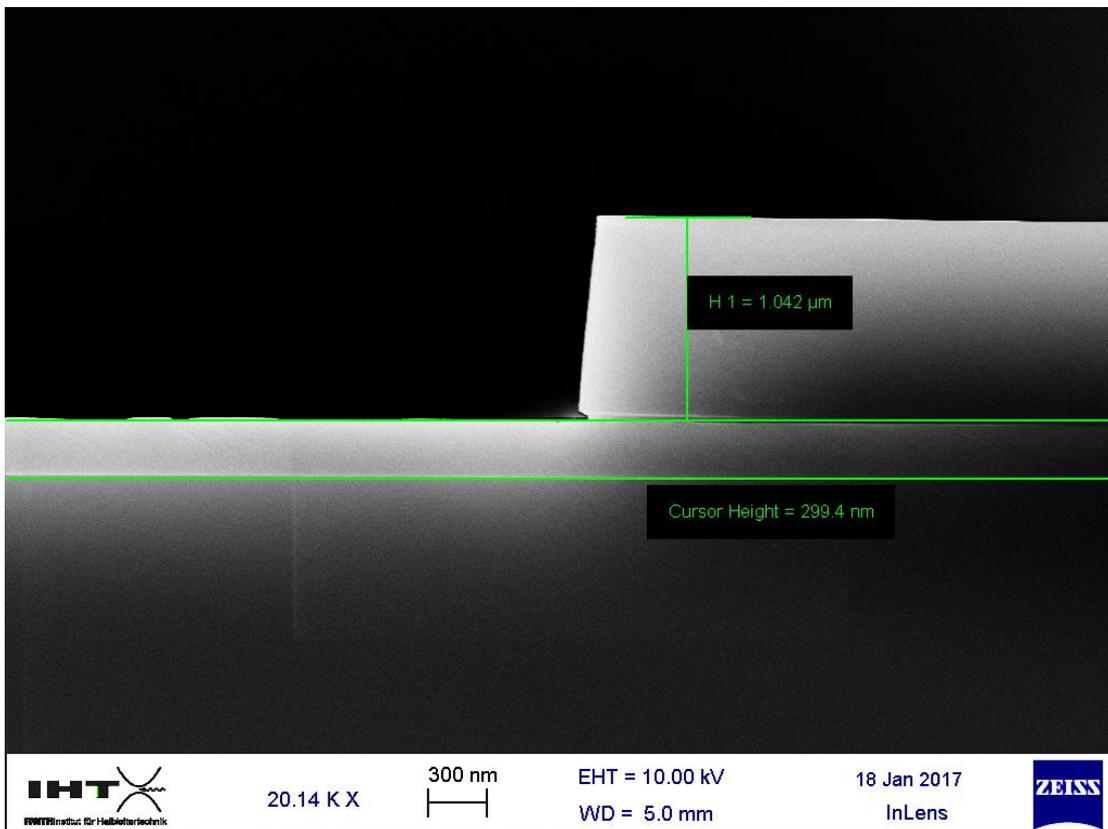
Figure 5. Etch profile of Alumina layer after Buffered Oxide Etching.
