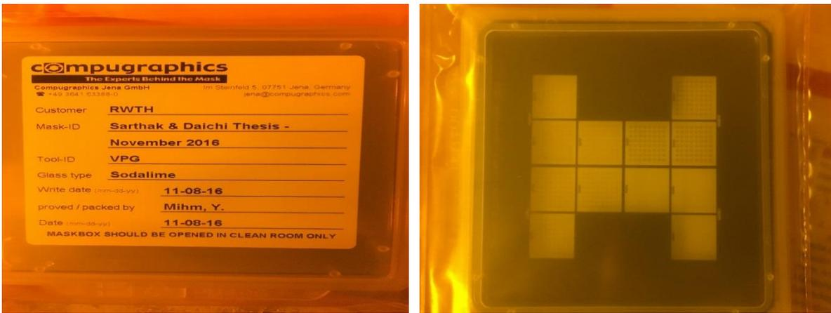
Figure 7. The Hard copy of the Mask showing four transparent region used for the device fabrication.
