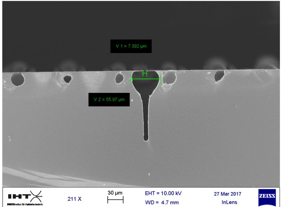
Figure 34. SEM image of the Opening of the trench after Strain Test 2
