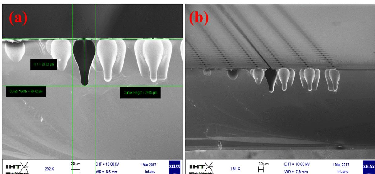
*Figure 22. (a) & (b) SEM of the Isotropic etching for 10 minutes*
