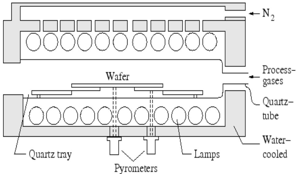
Figure 2.A schematic set-up of a Rapid Thermal Processing reactor
