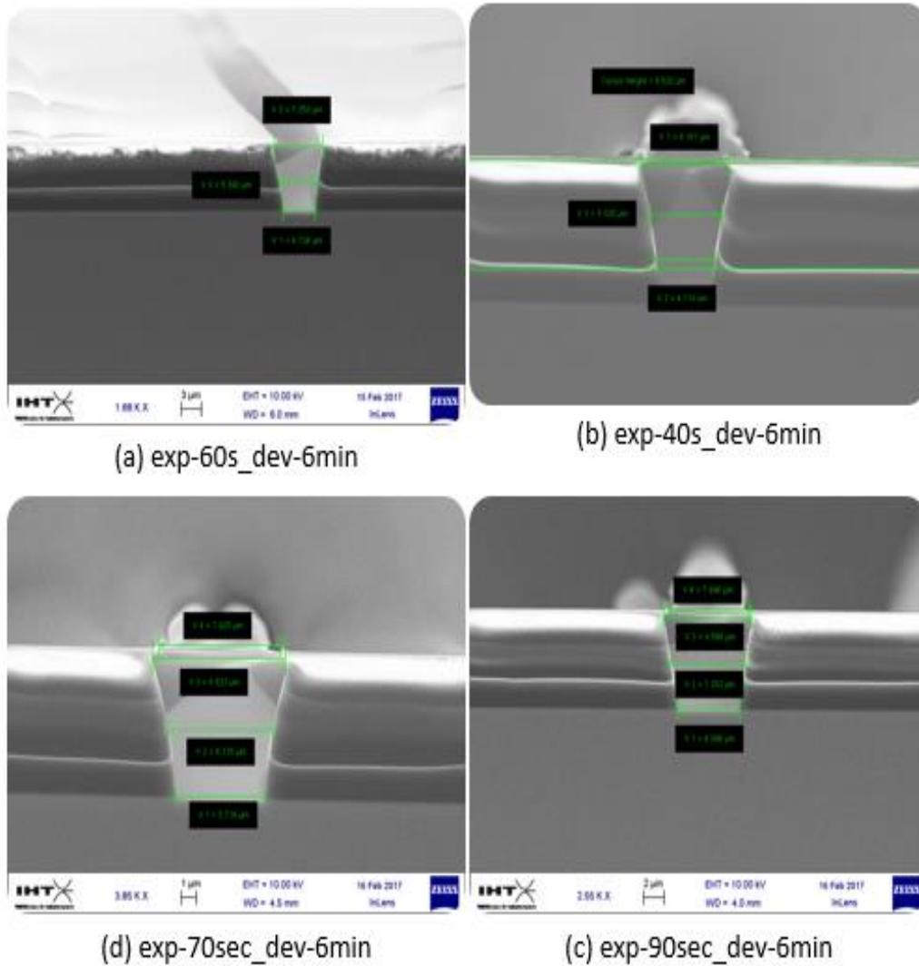
Figure 19. (a), (b), (c), & (d) showing results by altering the parameters for AZ9260 recipe
