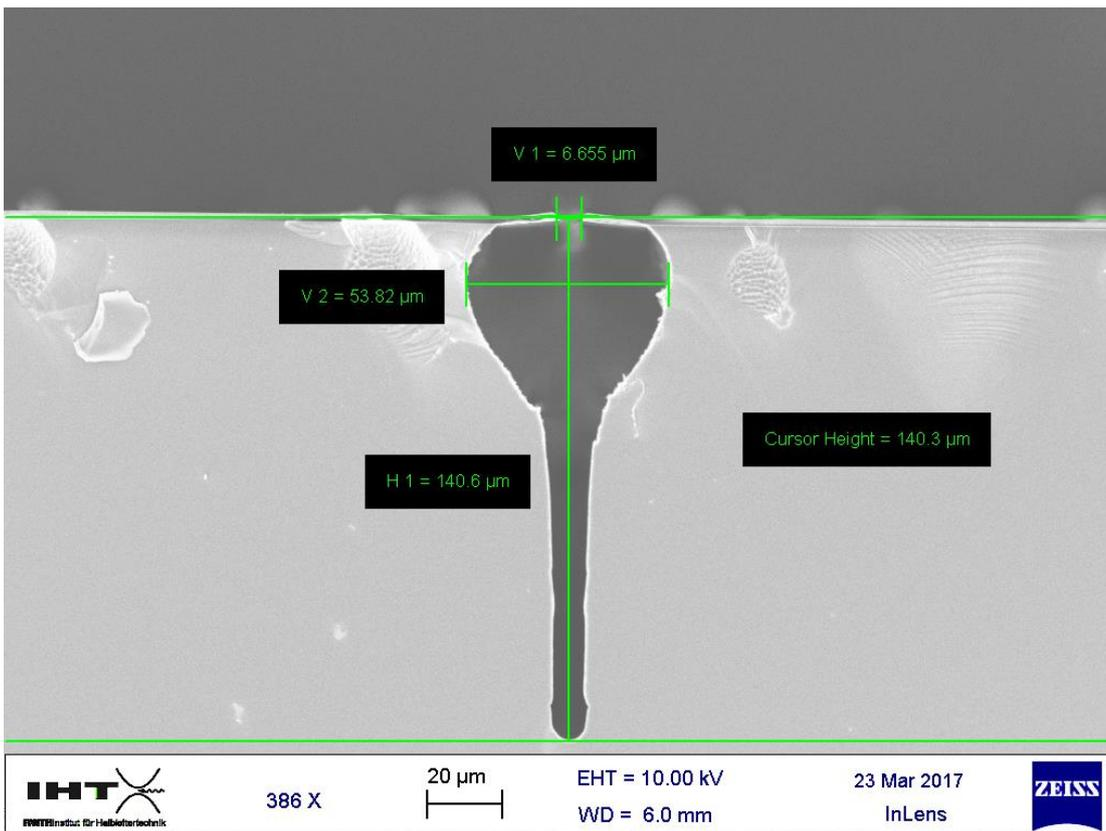
Figure 30. SEM image of the device showing the width of the opening before applying Strain
