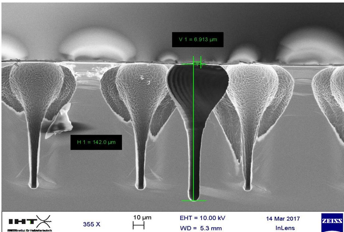
Figure 26. SEM image of etching profile after 45min Bosch + 10min Isotropic etch.
