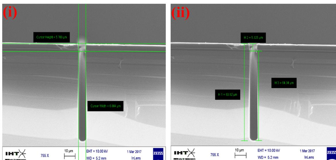
Figure 20. (i) & (ii) SEM image of Si etch into the substrate by HAR Bosch etching process
