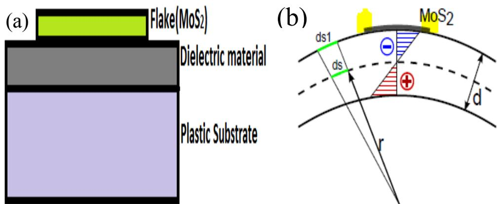
Figure 1. (a) A strain setup using plastic substrate. (b) Strained substrate.
