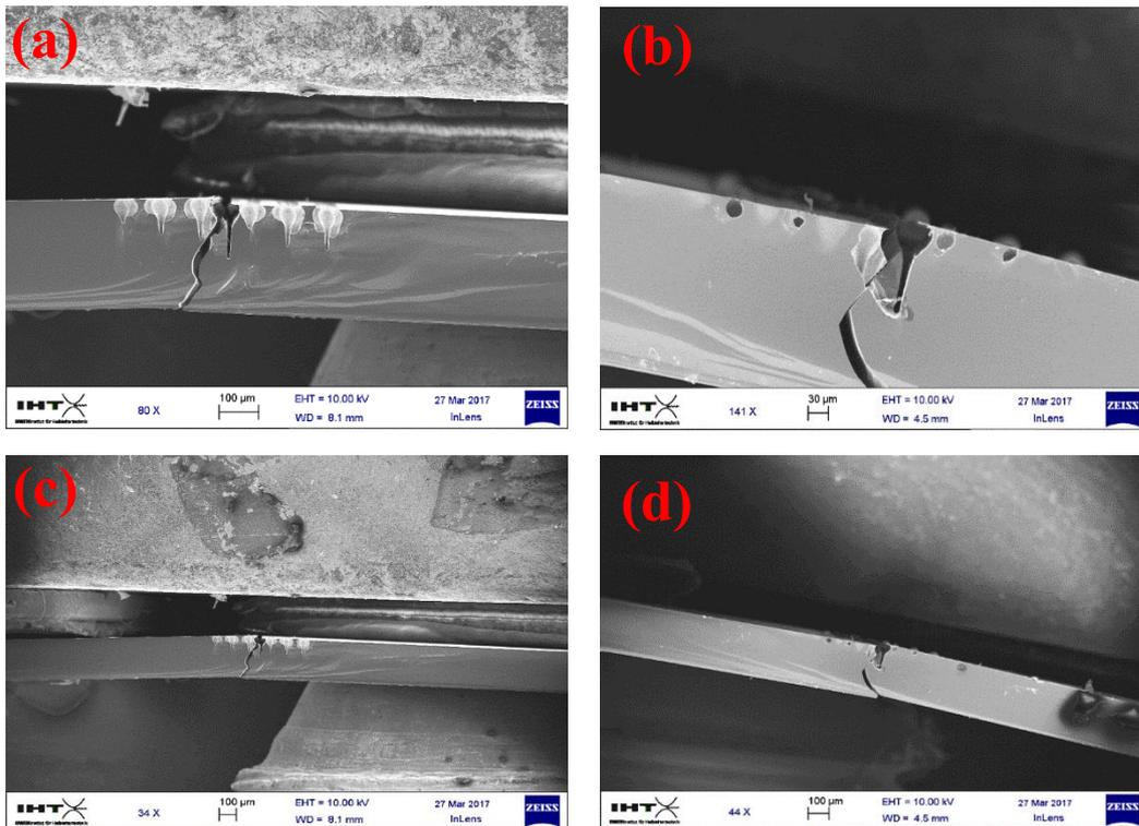
Figure 36. (a), (b), (c), (d) showing the breakdown of the device due to over strain in Test 4
