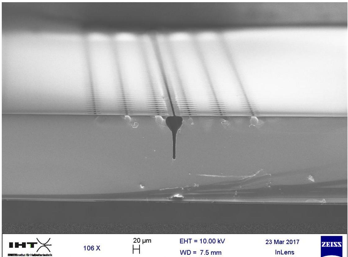
Figure 27. SEM image of the Final device fabricated using micro-electronic step
