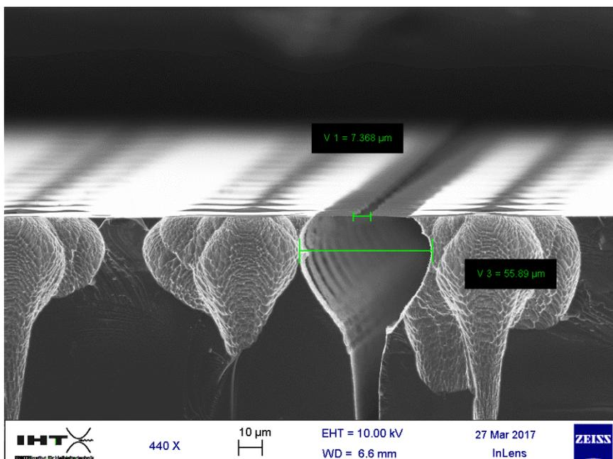
Figure 32. Straining effect on the opening of the trench after TEST 1.
