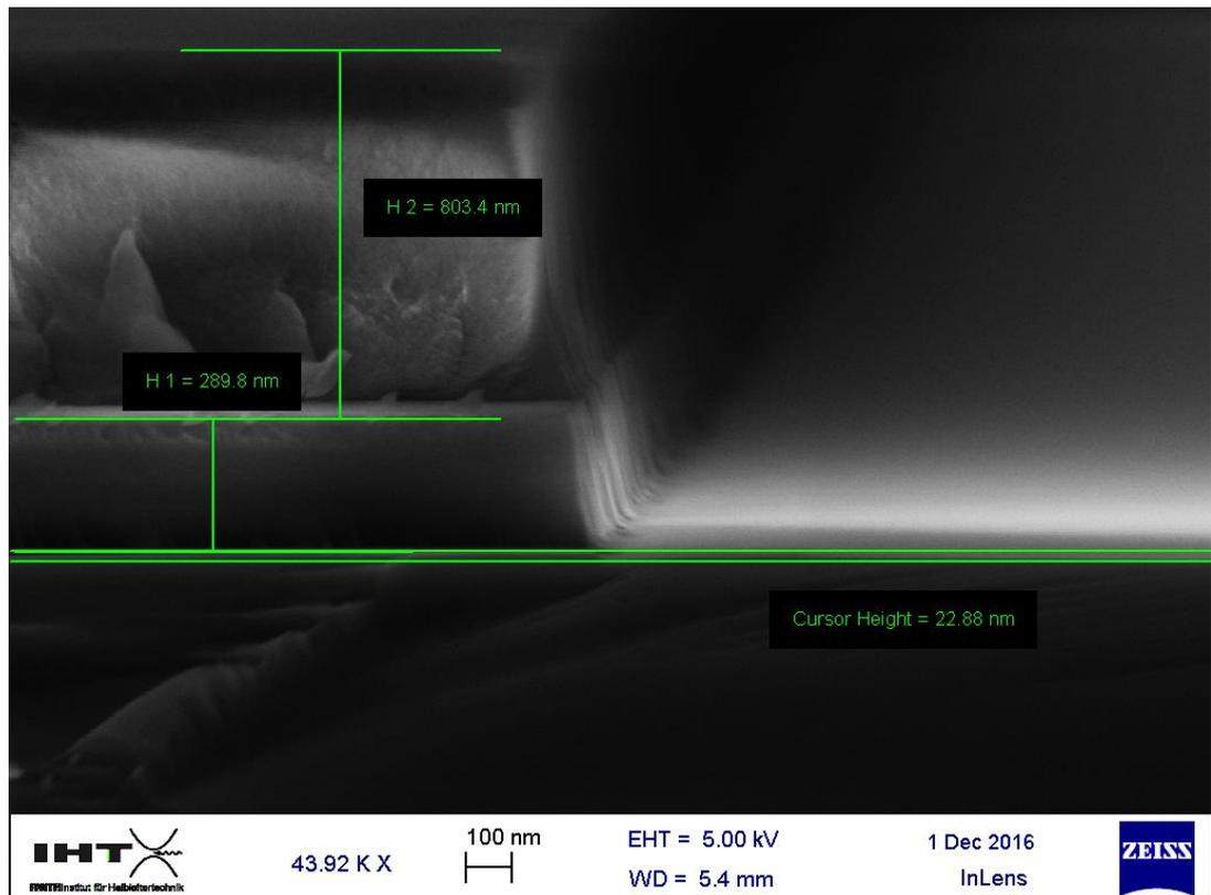
Figure 11. SEM image of the sample processed for 32 minutes in RIE 51
