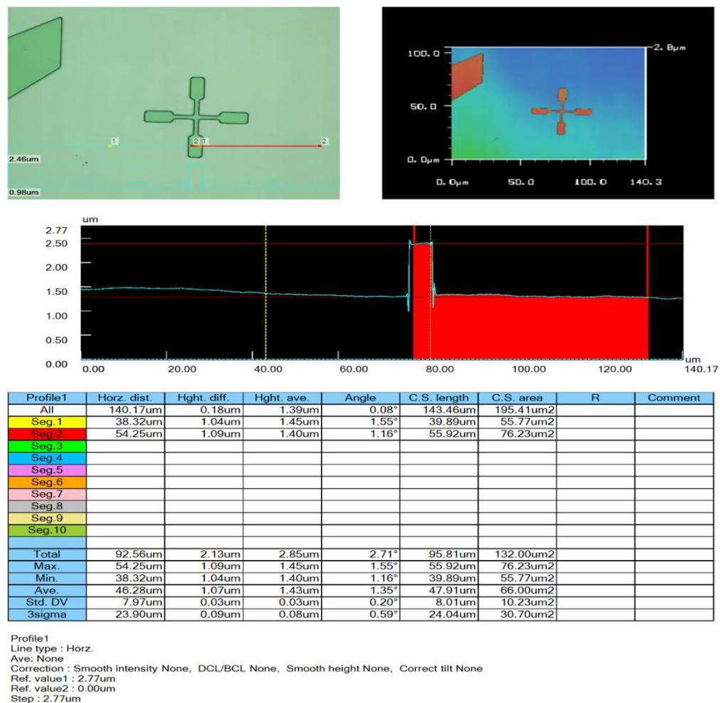
Figure 6. Etching Profile Measurement using Optical Laser Microscopy
