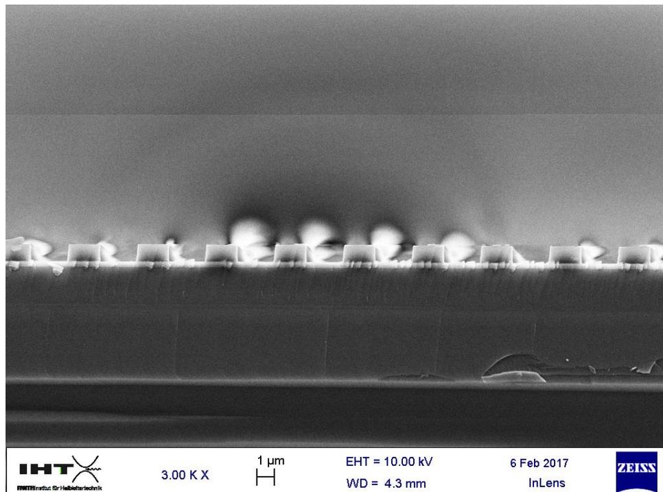
Figure 4. SEM Image of etching profile using Bosch process
