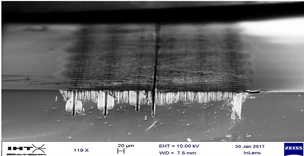
Figure 18. SEM image of the device fabricated using Method 2
