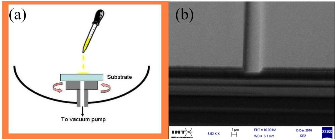
Figure 9. (a) Spin coating mechanism. (b) SEM image of uniform PR layer on Si Substrate
