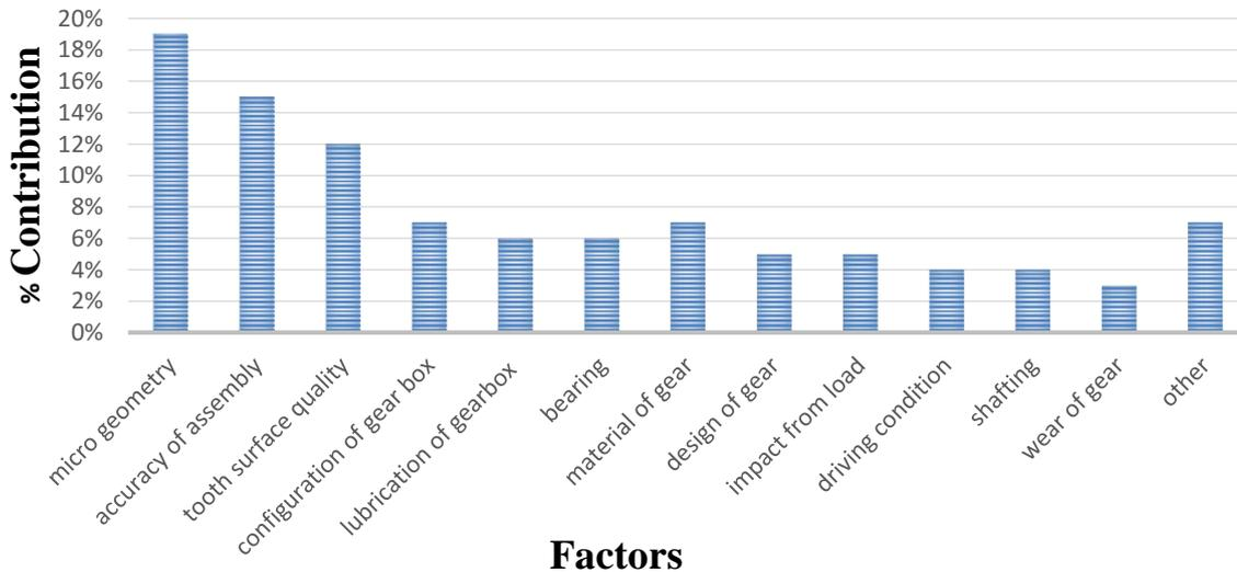
**Fig. 1.2:** Different factors contributing in noise and vibrations in a gear. (<http://khkgears.net/gear-knowledge/introduction-to-gears/gear-noise>).
