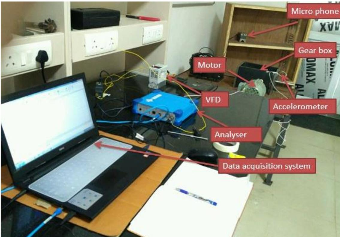
**Fig. 3.2:** Arrangement of the devices used to measure the noise and vibrations of spur gears.
