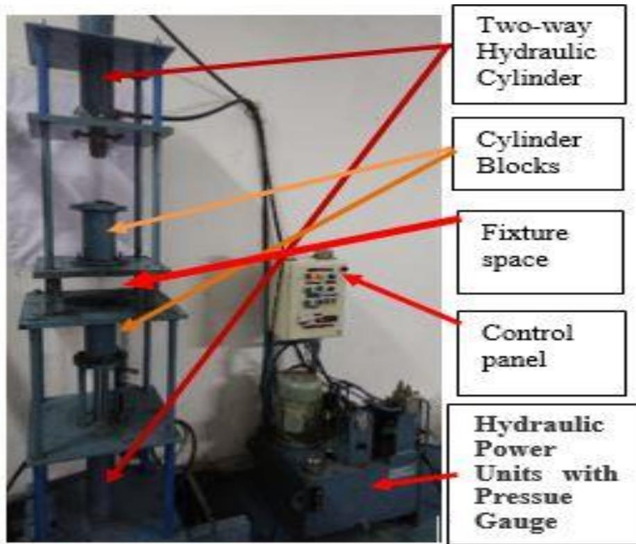
**Fig 4.1:** Photograph of AFF apparatus developed for gear finishing by Anand C Petare.
