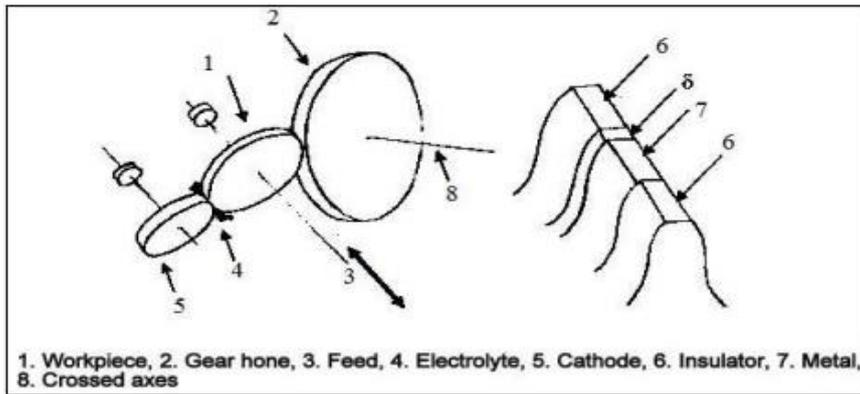
**Fig. 4.3:** Concept of finishing spur gears by ECH process proposed by **Chen et al. (1981)**.
