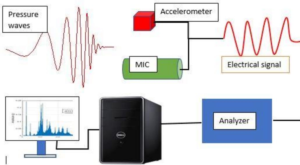
**Fig.1.3:** Flow chart of measurement of noise and vibrations.
