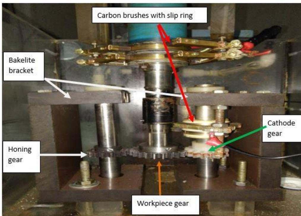
**Fig.4.4:** Photograph of the finishing chamber used for finishing spur gears by PECH.
