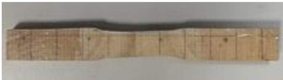
Fig. 4.7: Prepared specimen for double layer balsa wood composite material.
