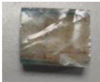
Fig. 4.11: Prepared compression specimen for single layer balsa wood composite material.
