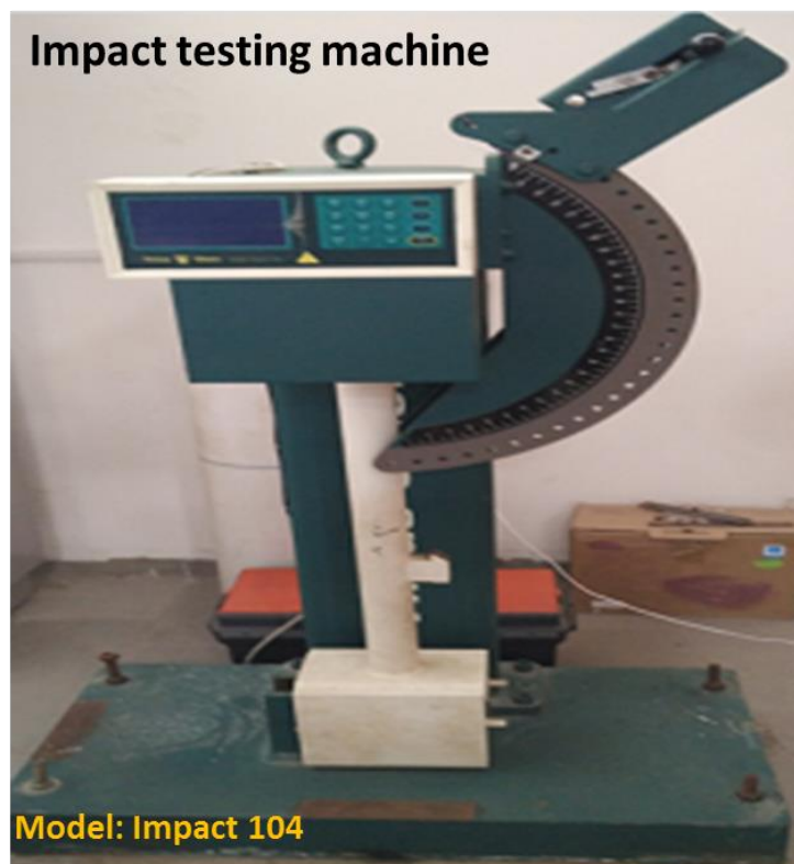
Fig. 4.18: Impact testing machine ( Model: Impact 104 from Tinius Olsen )
