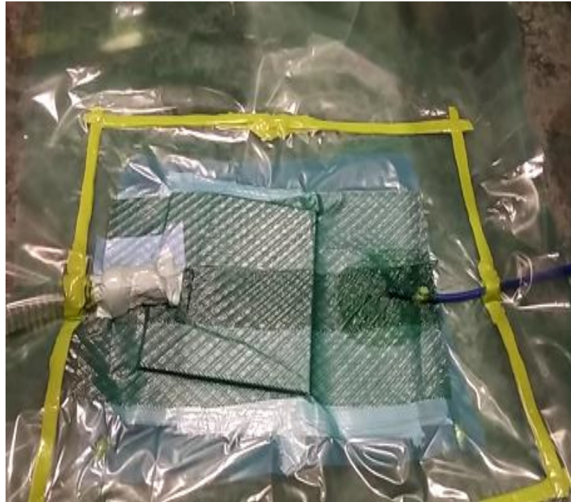
Fig. 3.3: Vacuum bag mold used to develop the composite material.
