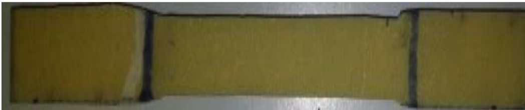
Fig. 4.3: Prepared specimen for single layer SAN foam composite material.
