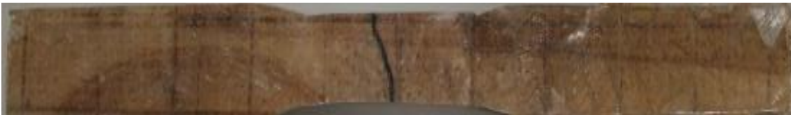
Fig. 4.9: Prepared specimen for single layer balsa wood composite material.
