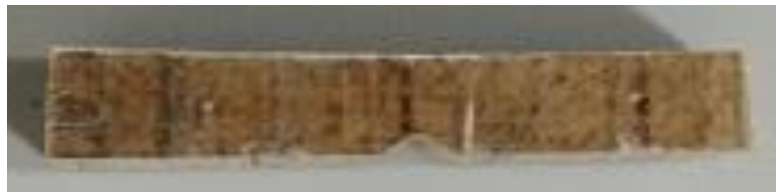
Fig. 4.21: Charpy test samples for balsa wood composite material.
