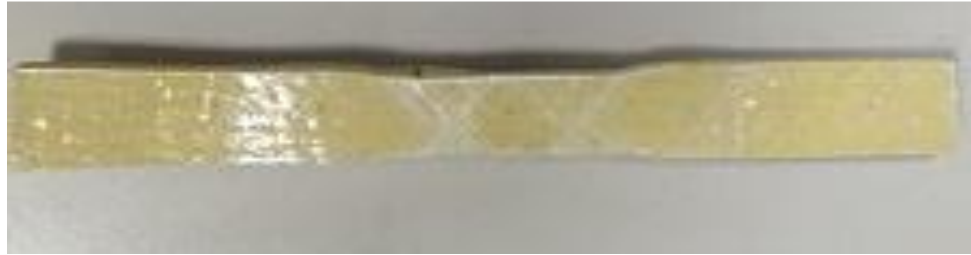
Fig. 4.5: Prepared specimen for double layer SAN foam composite material.
