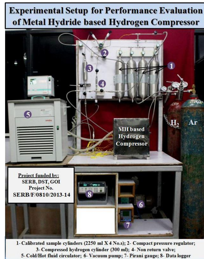
Fig. 4.2 (b) Experimental set up for performance measurement of MHC
