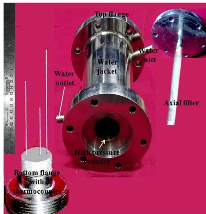
Fig. 4.3 (a) Schematic diagram of metal hydride bed for MHHC; (b) Components of metal hydride bed for MHHC
