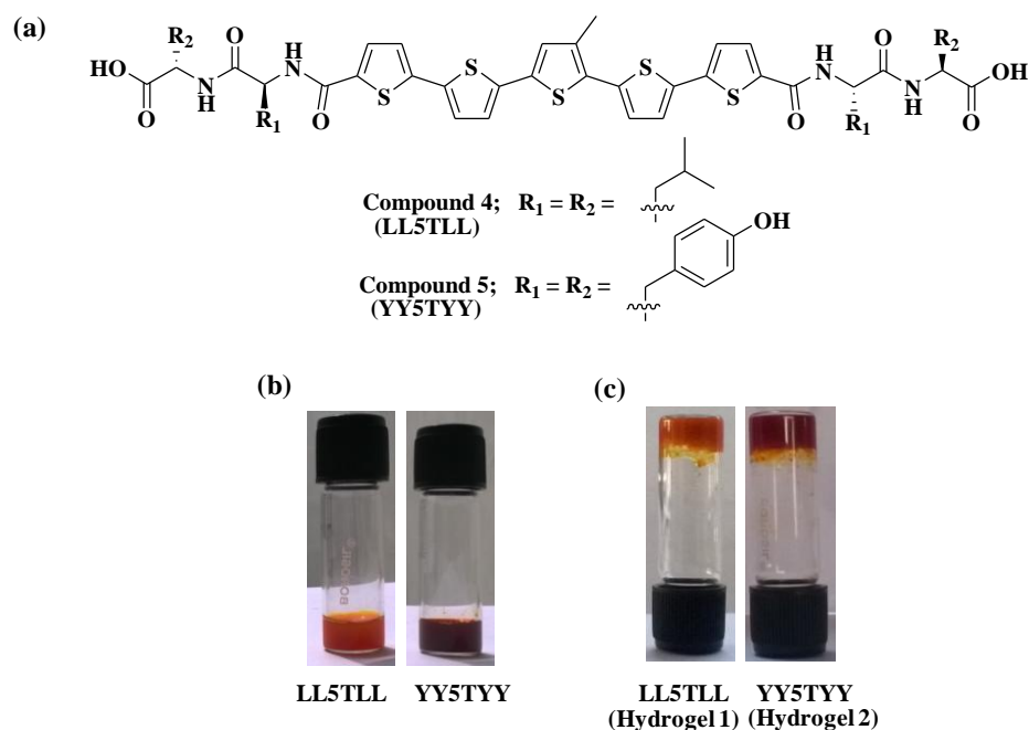
Figure 4.16. (a) Molecular structures of the peptide-quinquethiophene conjugates 4 (LL5TLL) and, 5 (YY5TYY); (b) Digital images of the solution of compounds 4 and 5 at basic pH and (c) hydrogel 1 and 2 .
