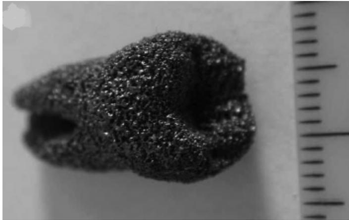
**Fig.2.6**3D NiTi structures developed by SLS [Shishkovsky et al 2008]
