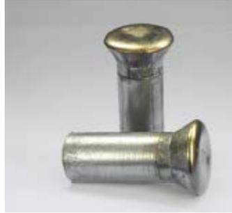
**Fig.2.10** Bulk NiTi ingots developed by SLM [Habijan et al.2013]
