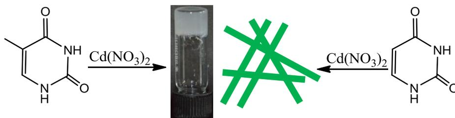
**Scheme 7.1.** Schematic for the generation of coordination polymer hydrogel using T and U as ligands and  $\text{Cd}(\text{NO}_3)_2$  as metal salt.
