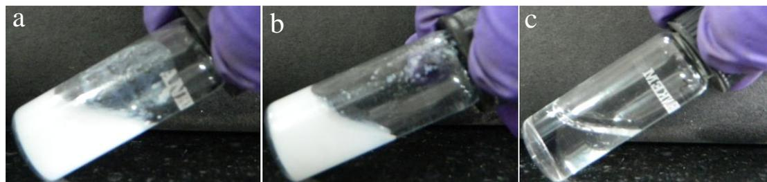
**Figure 7.5.** Digital images of (a) Cd-A precipitate, (b) Cd-G precipitate and (c) Cd-C clear solution respectively.
