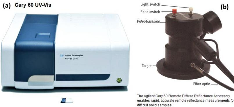
**Fig.(2.5):** Experimental set up for diffuse reflectance measurement (a)Cary 60 UV-Vis spectrometer, (b) an integrating sphere attachment to detect diffuse reflectance.
