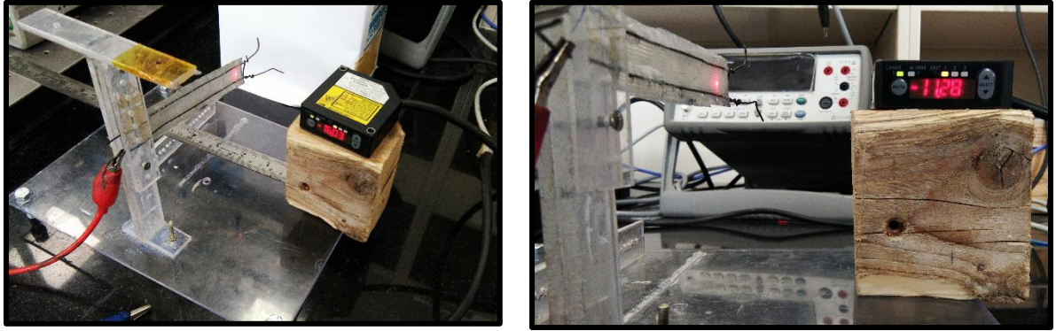
Figure 21 Deflection analysis of Epoxy structure
