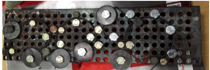
Figure 15 Fixture for Training SMA
