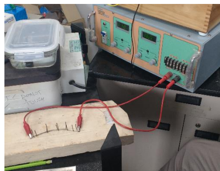
Figure 16 Training SMA through Joules Heating
