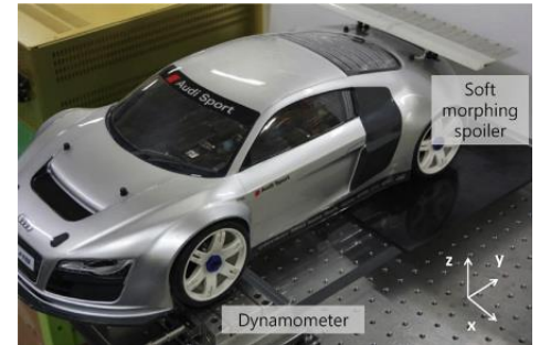
Figure 10 Morphing spoiler with small scale car [1]
