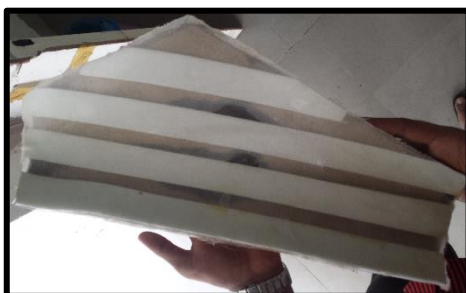
Figure 26 Curing of Smart blade
