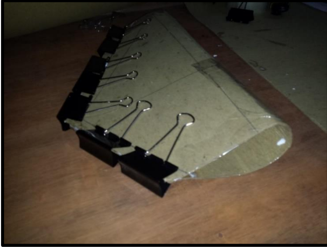
Figure 24 Cardboard mould for Wax pattern
