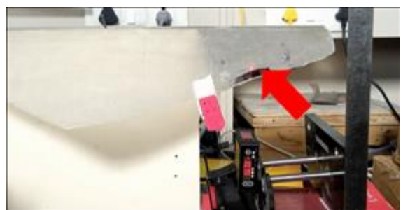
Figure 31 SMA Spring actuated Blade
