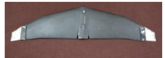
Figure 12 UAV with the mounted morphing winglets Top view [4] .
