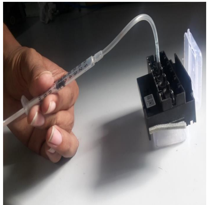
Fig. 8 - Cleaning Print head with VMS cleaning
